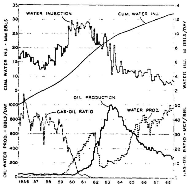
Fig. 11—Chimney Hill pilot waterflood performance.
