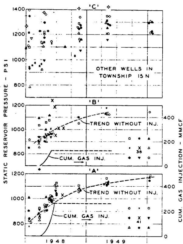
Fig. 4—Reservoir pressure buildup—Twp 15N pilot gas injection test No. 3, Bois d'Arc.
