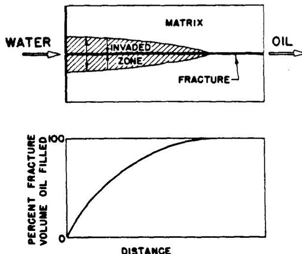
**Fig. 2—Illustration of Oil Production by Water Imbibition**
