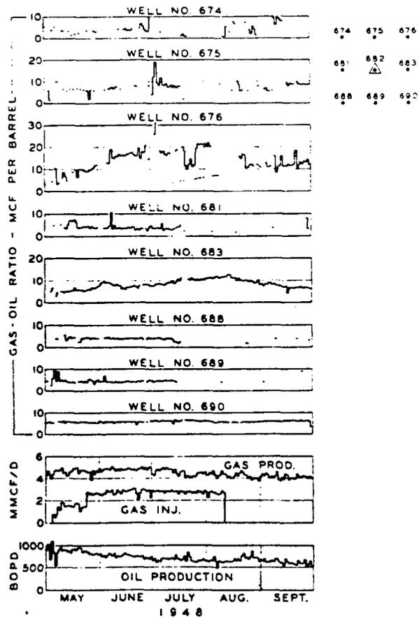
Fig. 5—Pilot gas injection test No. 1, Bois d'Arc.
