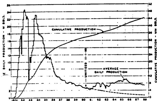
Fig. 2—Primary production and waterflood performance, Spraberry Driver Unit.
