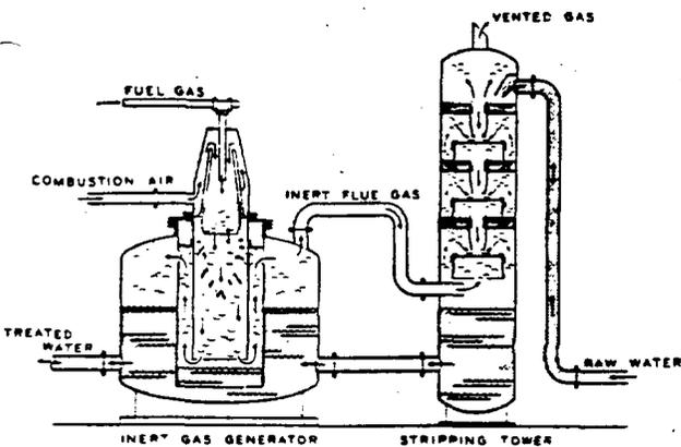
Fig. 8—Schematic diagram of water sweetening plants, Spraberry Driver Unit.
