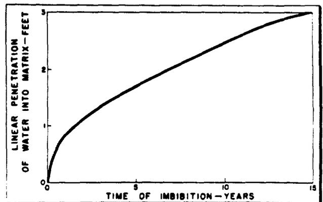
Fig. 5—Estimated Linear Advance of the Water Front with Imbibition under Spraberry Reservoir Conditions
