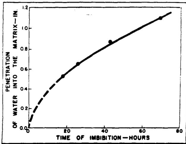
Fig. 4—Penetration of Water in Spraberry Matrix in Laboratory Imbibition-displacement Experiment
