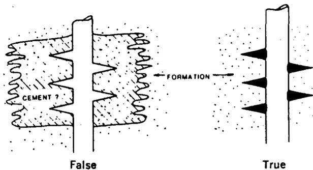
Fig. 9.10 Misconception 1 — Whole cement is squeezed into formation.<sup>11</sup>
