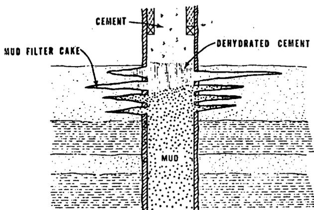
Fig. 9.8 Slurry dehydration across open perforations during a high-pressure squeeze operation.
