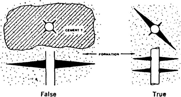
Fig. 9.12 Misconception 3 — Squeezing produces a horizontal pancake of cement.<sup>11</sup>
