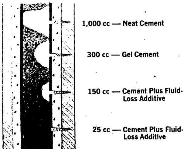
Fig. 9.9 Cement node buildup effect with filtration control (showing API fluid loss in cc/30 minutes at 1,000 psi).
