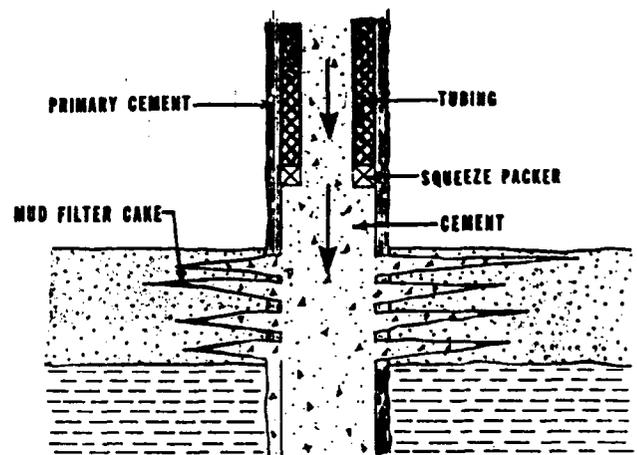
Fig. 9.1 Typical squeeze operation (packer set above perforations to control pressures and flow of cement slurry to formation).
