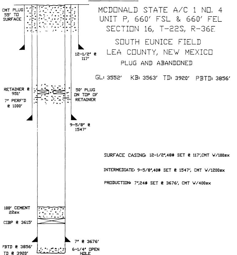
HISTORY: THE MCDONALD STATE A/C 1 NO. 4 WAS DRILLED AND COMPLETED IN MARCH, 1936. IP 35 BOPD, 0 BWPD AND 25 MCFD. 3/38 WELL WAS PLUGGED BACK FROM 3920' TO 3856' IN OCTOBER, 1962 THIS WELL WAS P&A'D AS FOLLOWS: SET CAST IRON BRIDGE PLUG IN 7" CASING @ 3615'. SPOTTED 100' CMT PLUG FROM 3615' TO 3515' W/22sx. PERF'D 7" @ 1000'. SET CAST IRON CEMENT RETAINER @ 951'. CMT W/200sx AND HAD GOOD CEMENT RETURNS TO SURFACE, SPOTTED CEMENT PLUG FROM 55' TO SURFACE, CUT OFF 7" AND INSTALLED WELL MARKER.
