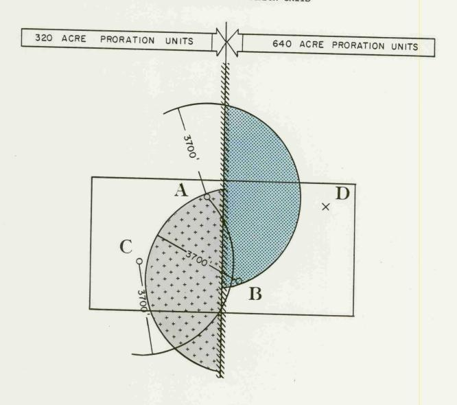
IF WELL B IS DRILLED AS SE DIAGONAL OFFSET TO WELL A, IT MUST COMPETE WITH WELL C FOR DRAINAGE OF AREA WEST OF BOUNDARY.
