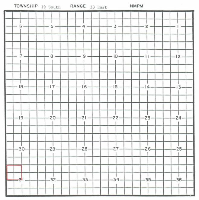
Mitchell Energy Corporation Geronimo Federal Well No. 1 located in Unit D of Section 31, Township 19 South, Range 33 East, NMPM. It was completed October 3, 1990, in the Delaware formation. The top of the perforations is at 7,586 feet.
