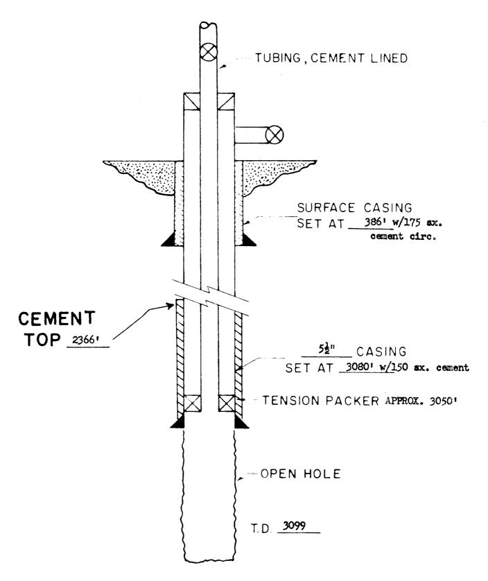
WATER INJECTION WELL SCHEMATIC
