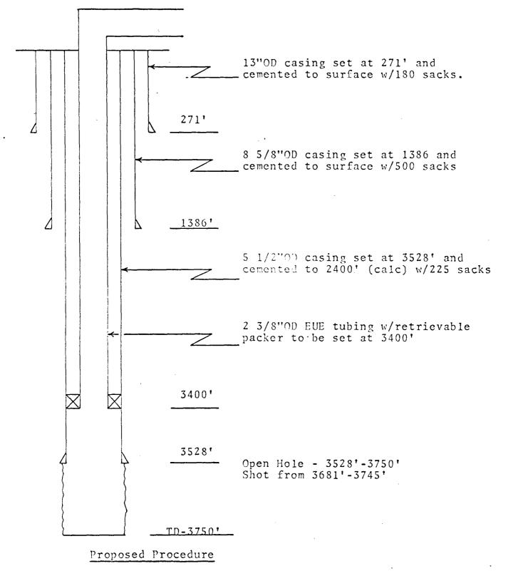
Tag bottom - tally out. Clean out to TD. Run tubing w/packer to be set at 3400'. Connect up well for injection down tubing. 1.
