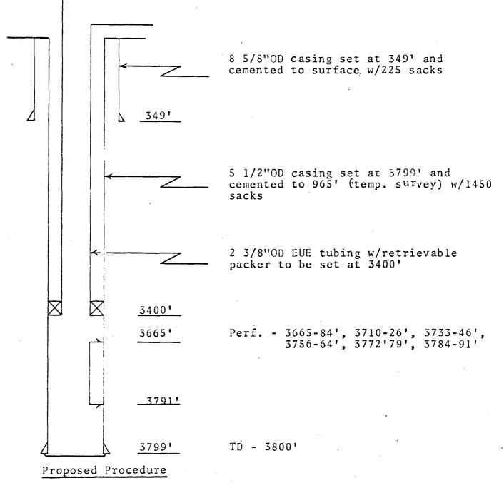
Tag bottom & tally out. Clean out to 3795' Run tubing w/packer to be set at 3400' Connect up well for injection down tubing. 1.
