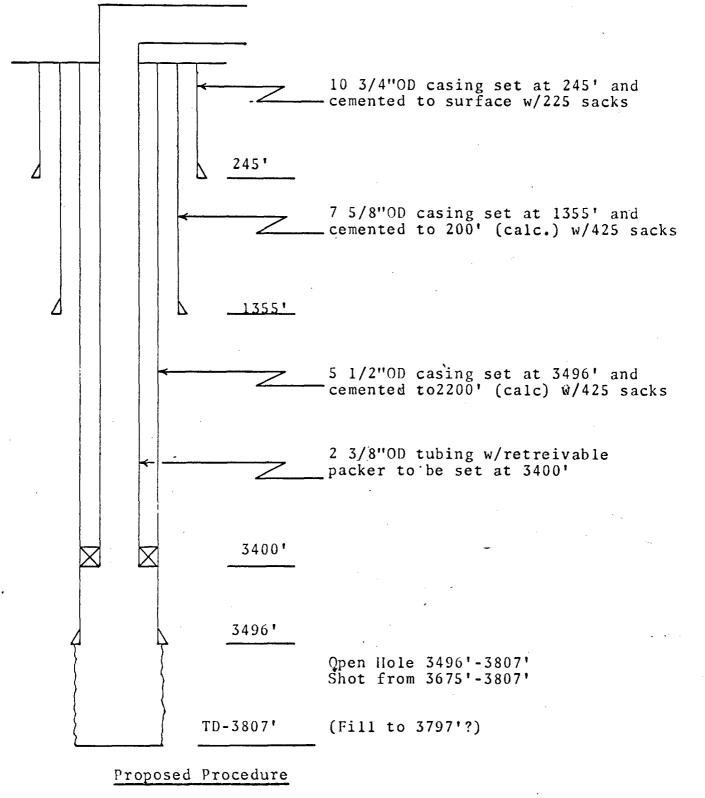
Tag bottom tally out. Clean out to 3807' Run tubing w/packer to be set at 3400' Connect up well for injection down tubing. 1.
