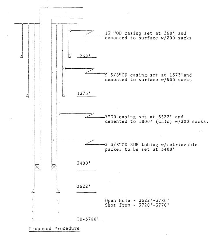
Tag bottom - tally out. Clean out to 3775'. Run tubing w/packer to be set at 3400' Connect up well for injection down tubing. 1.
