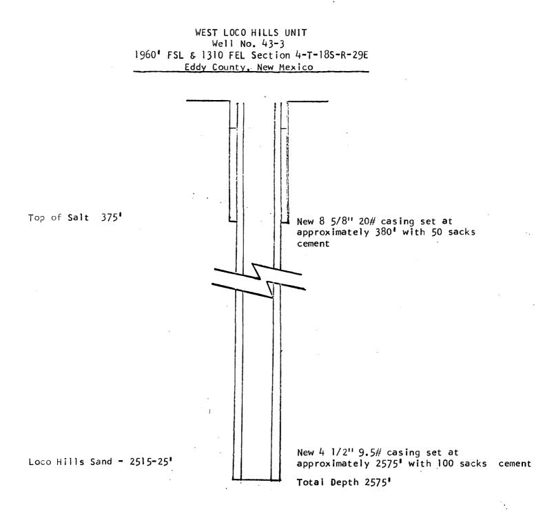
Water to be injected down casing through perforations at approximately 2515-25"
