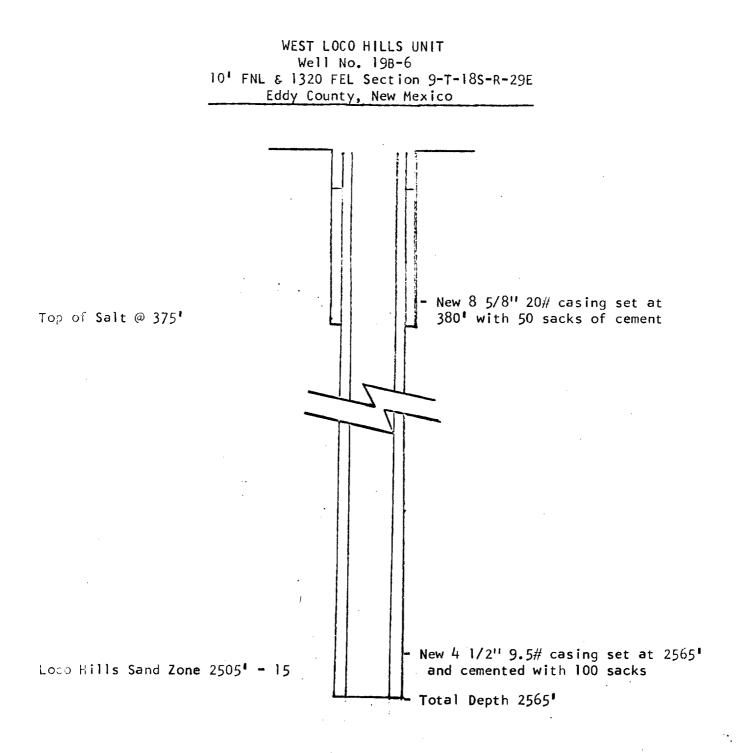
Water to be injected down casing through perforations at approximately 2505-15
