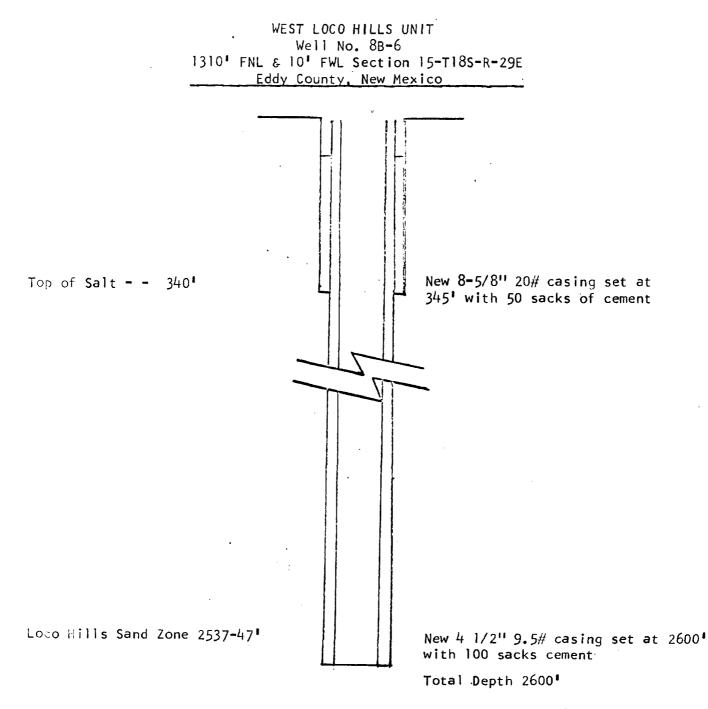
Water to be injected down casing through perforations at 2537-47\*
