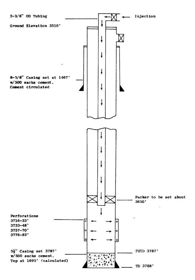
Schematic Drawing of Injection Well
