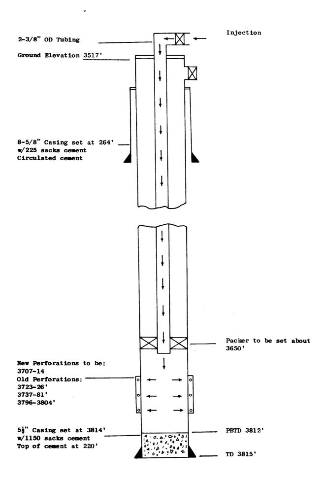
Schematic Drawing of Injection Well
