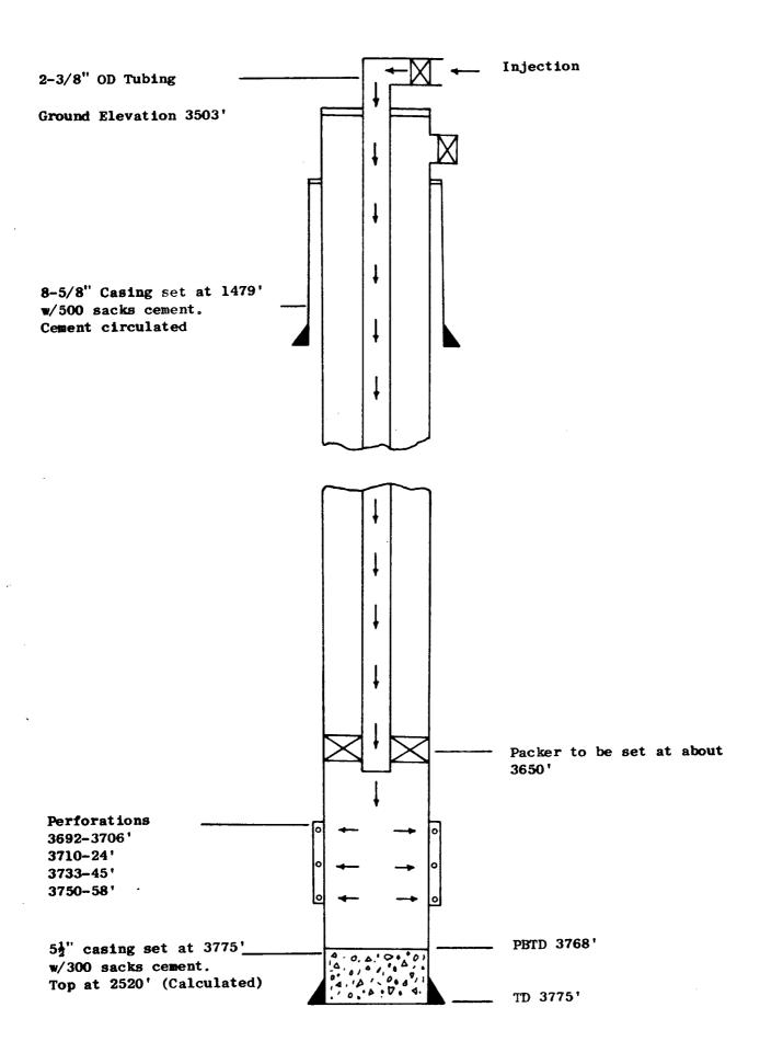
Schematic Drawing of Injection Well
