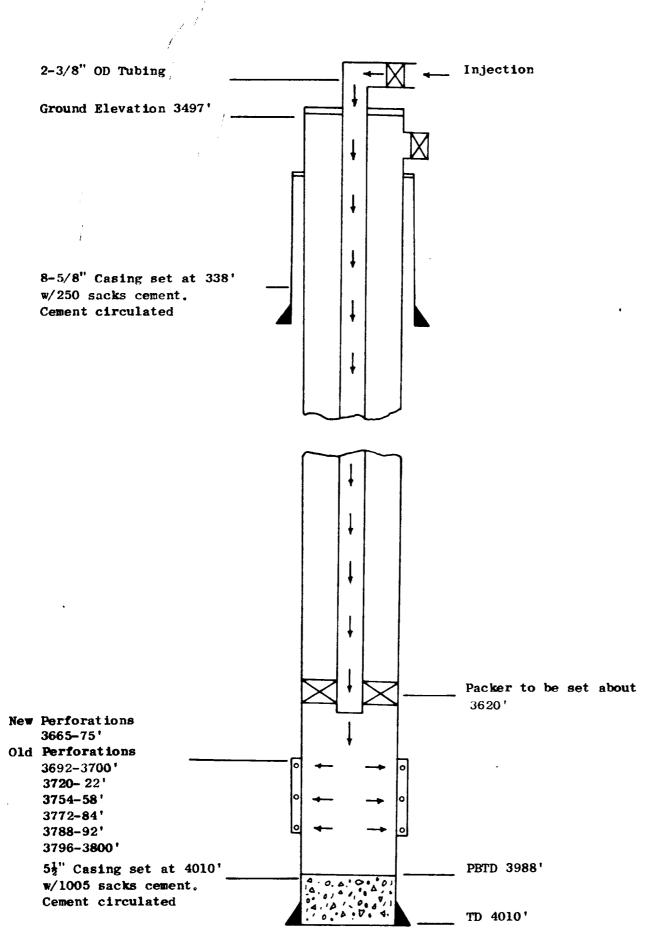
Schematic Drawing of Injection Well
