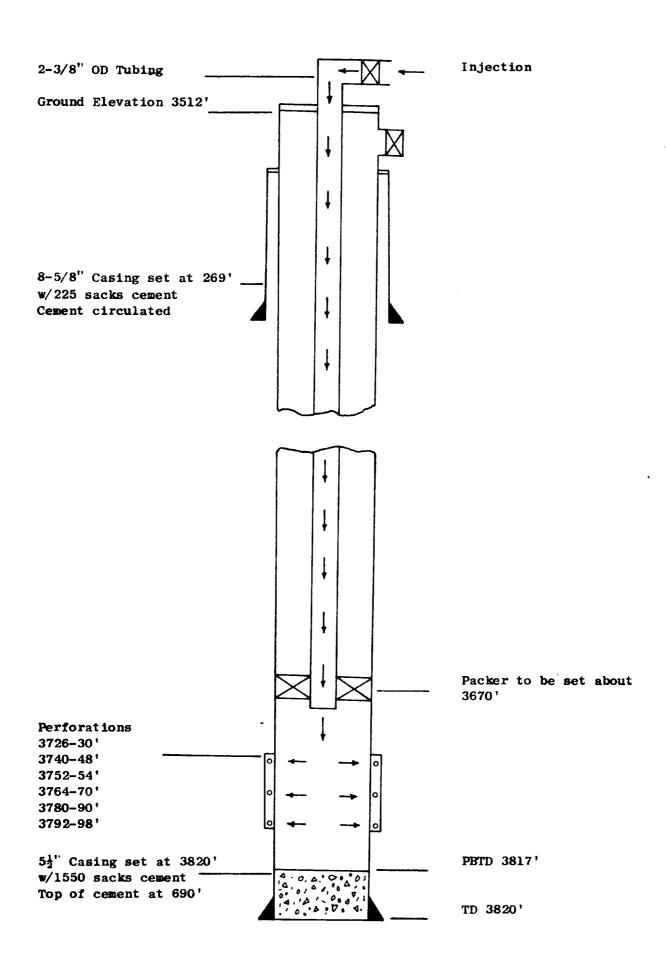
Schematic Drawing of Injection Well
