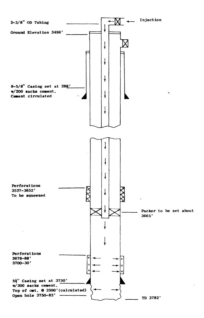
Schematic Drawing of Injection Well
