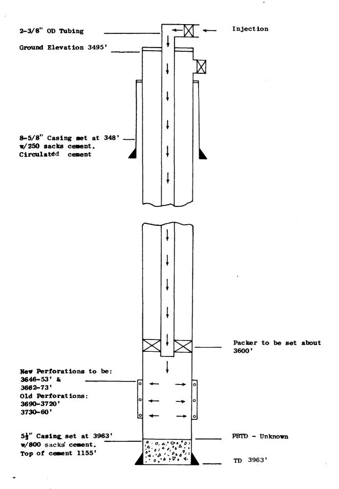
Schematic Drawing of Injection Well
