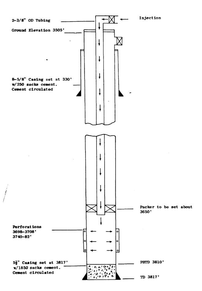
Schematic Drawing of Injection Well
