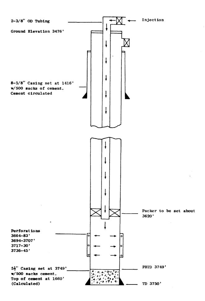
Schematic Drawing of Injection Well Unit Well No. 23 (ARCo C. Jones No. 9) 1980' FNL & 660' FWL Section 34, T-22S, R-36E Lea County, New Mexico
