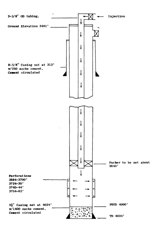
Schematic Drawing of Injection Well
