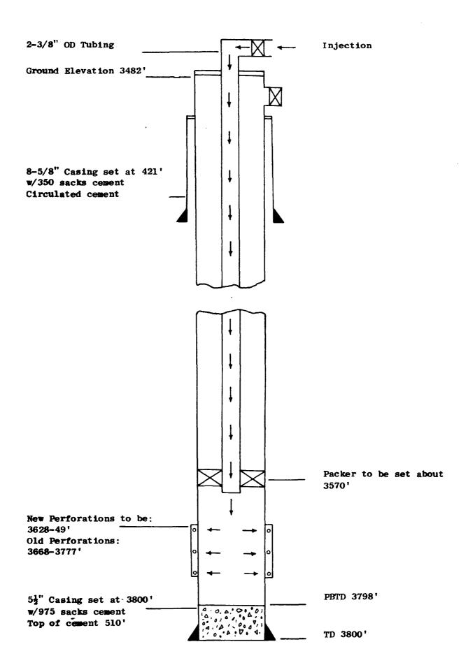
Schematic Drawing of Injection Well
