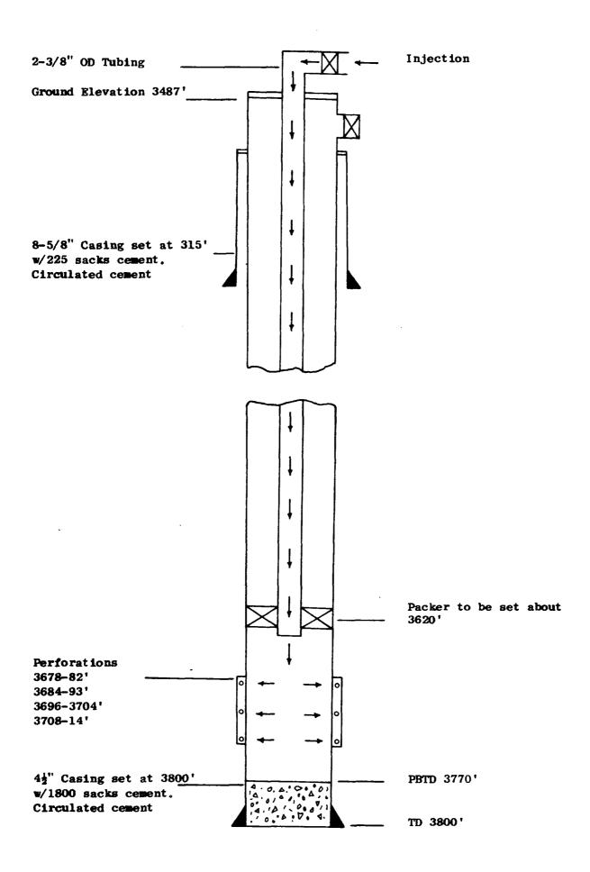
Schematic Drawing of Injection Well
