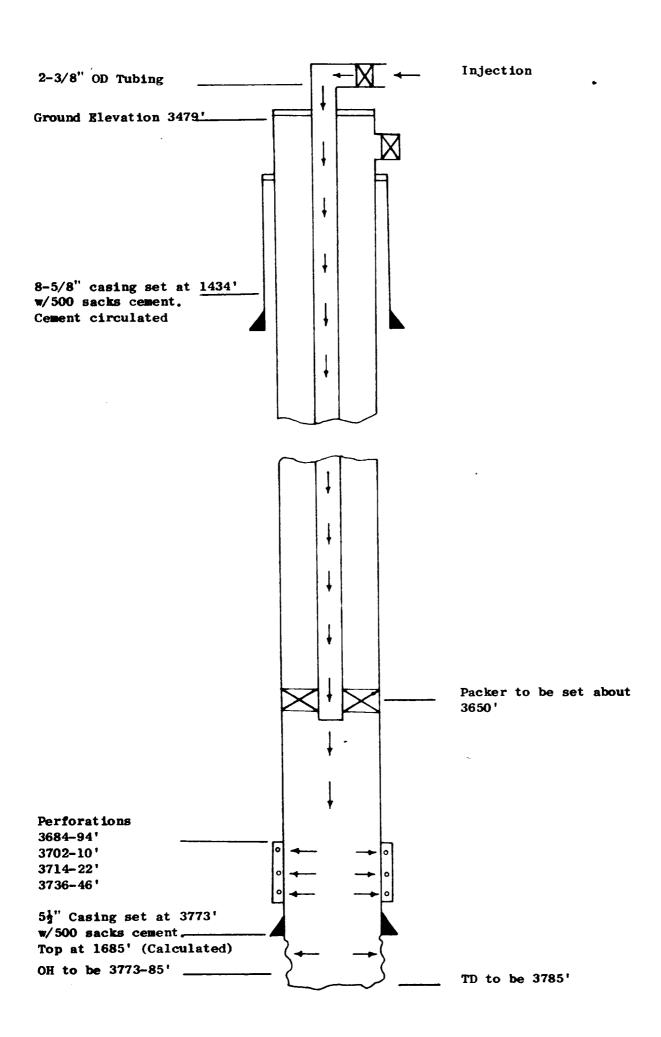
Schematic Drawing of Injection Well
