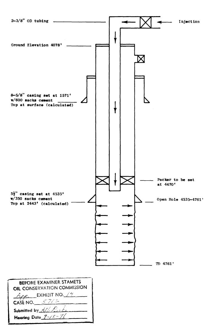
ATLANTIC RICHFIELD COMPANY STATE VACUUM UNIT Schematic Drawing of Injection Well Unit Well No. 19 (A.R.Co. State "C" TG No. 5) 990' FSL & 1650' FEL Section 32, T-17S, R-34E Lea County, New Mexico
