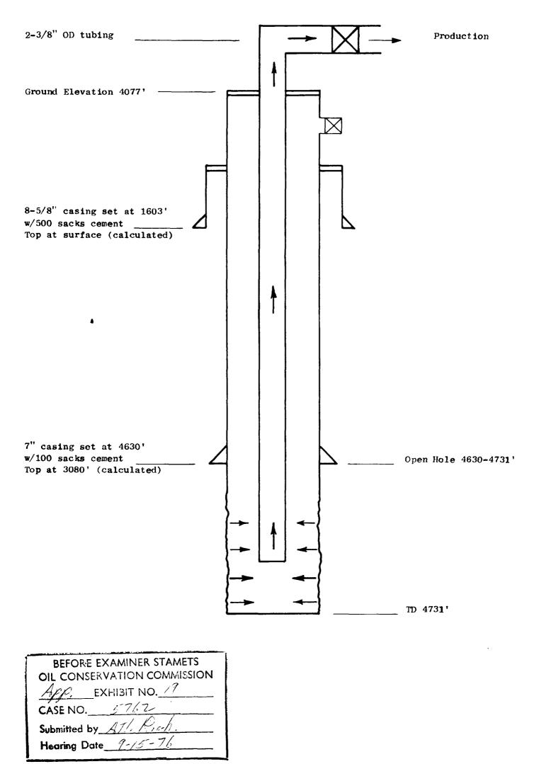
ATIANTIC RICHFIELD COMPANY STATE VACUUM UNIT Schematic Drawing of Producing Well Unit Well No. 8 (A.R.Co. State "B" TG No. 2) 1980' FNL & 1980' FWL Section 32, T-17S, R-34E Lea County, New Mexico
