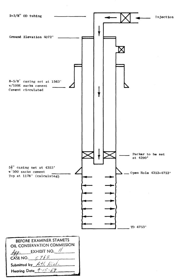
ATLANTIC RICHFIELD COMPANY STATE VACUUM UNIT Schematic Drawing of Injection Well Unit Well No. 13 (A.R.Co. State "C" TG No. 3) 1980' FSL & 1980' FWL Section 32, T-17S, R-34E Lea County, New Mexico
