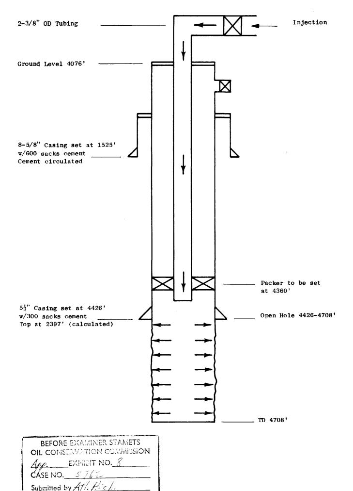
ATIANTIC RICHFIELD COMPANY STATE VACUUM UNIT Schematic Drawing of Injection Well Unit Well No. 7 (A.R.Co. State "B" TG No. 3) 1980' FNL & 660' FWL Section 32, T-17S, R-34E Lea County, New Mexico
