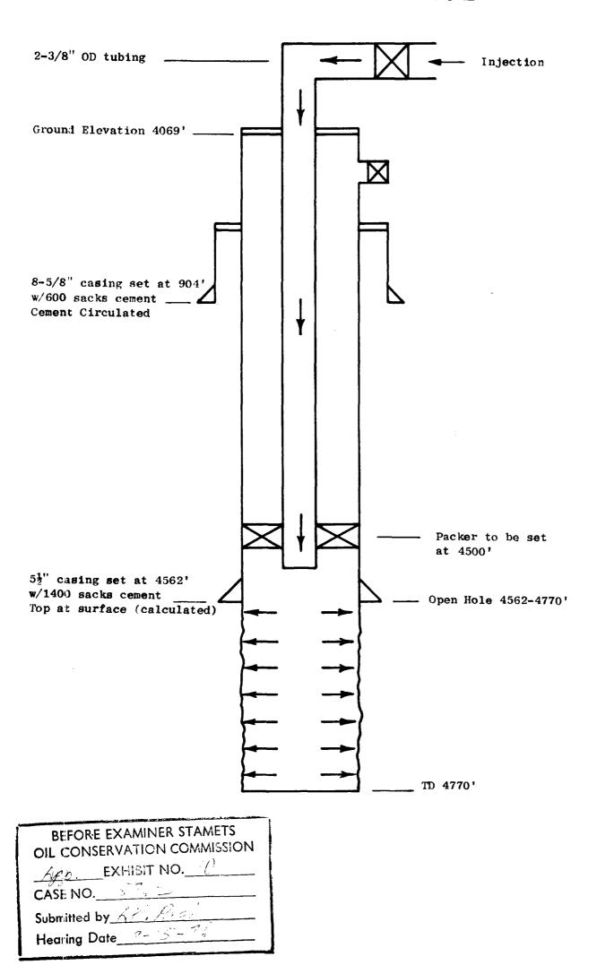
ATLANTIC RICHFIELD COMPANY STATE VACUUM UNIT Schematic Drawing of Injection Well Unit Well No. 11 (Texaco New Mexico "AO" State No. 1) 2310' FSL & 330' FEL Section 31. T-17S. R-34E Lea County, New Mexico
