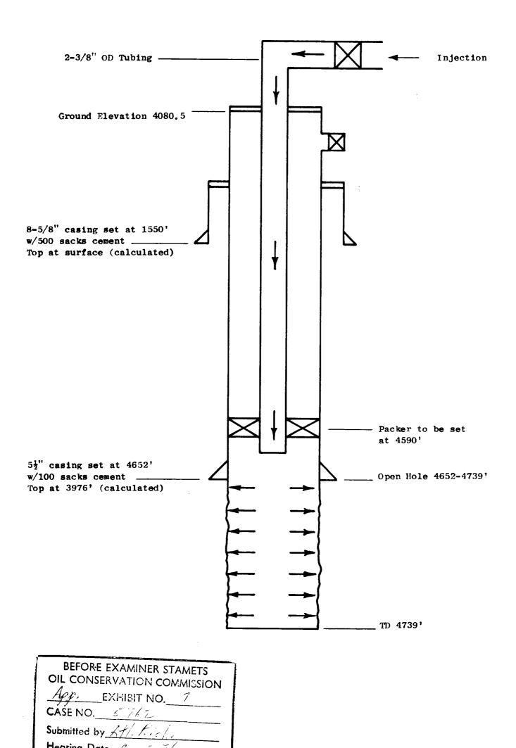
ATLANTIC RICHFIELD COMPANY STATE VACUUM UNIT Schematic Drawing of Injection Well Unit Well No. 4 (A.R.Co. State "B" TG No. 4) 990' FNL & 1650' FWL Section 32, T-17S R-34E Lea County, New Mexico
