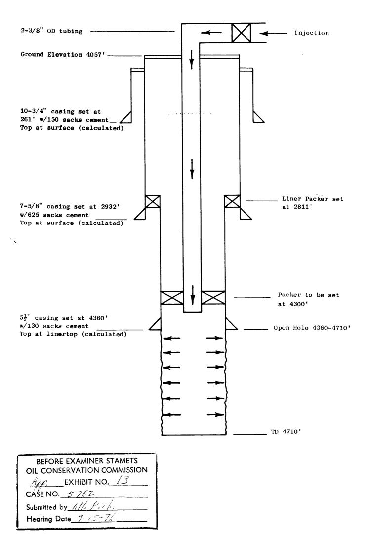
ATLANTIC RICHFIELD COMPANY STATE VACUUM UNIT Schematic Drawing of Injection Well Unit Well No. 17 (A.R.Co. State "C" TG No. 8) 990' FSL & 990' FWL Section 32, T-17S, R-34E Lea County, New Mexico
