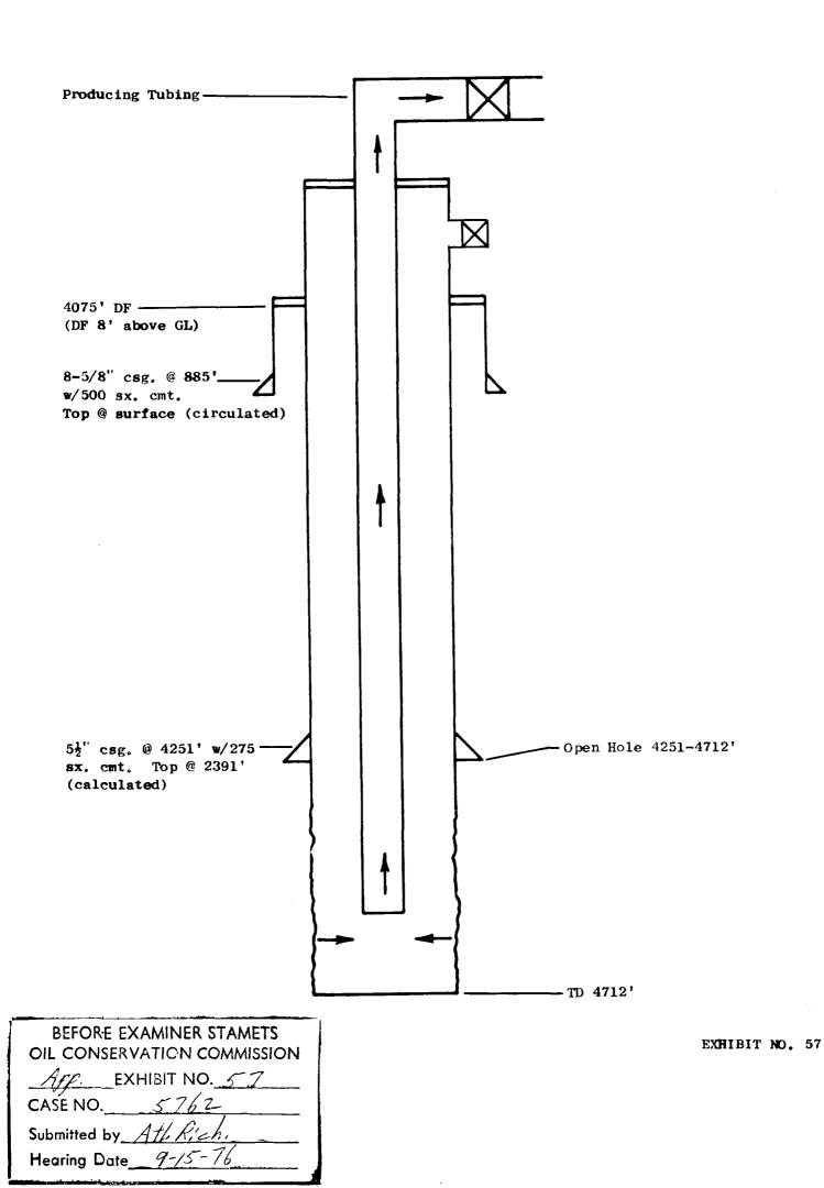
TEXACO - WEST VACUUM UNIT NO. 31) (Texaco - State of New Mexico "O" NCT-2 #17) Unit N 660' FSL & 1980' FWL Section 33, T-17S, R-34E
