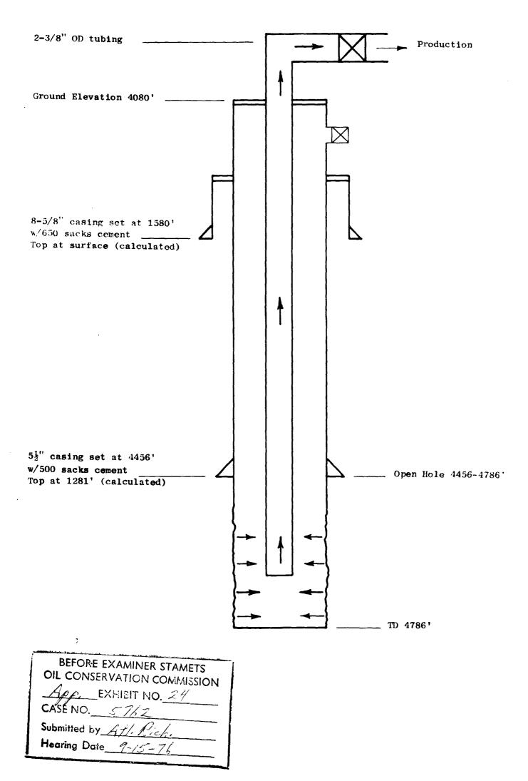
ATLANTIC RICHFIELD COMPANY STATE VACUUM UNIT Schematic Drawing of Producing Well Unit Well No. 20 (A.R.Co. State "C" TG No. 4) 660' FSL & 660' FEL Section 32, T-17S, R-34E Lea County, New Mexico
