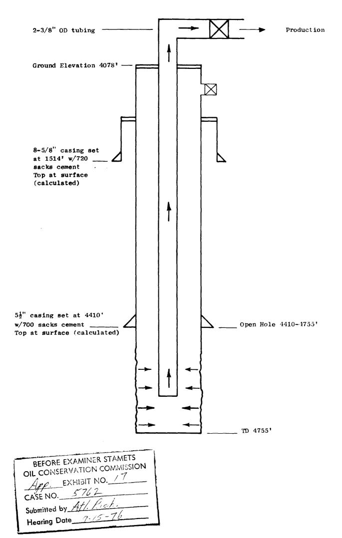
ATLANTIC RICHFIELD COMPANY STATE VACUUM UNIT Schematic Drawing of Producing Well Unit Well No. 5 (Texaco New Mexico "D" State NCT-2 No. 4) 990' FNL & 2310' FEL Section 32, T-17S, R-34E Lea County, New Mexico
