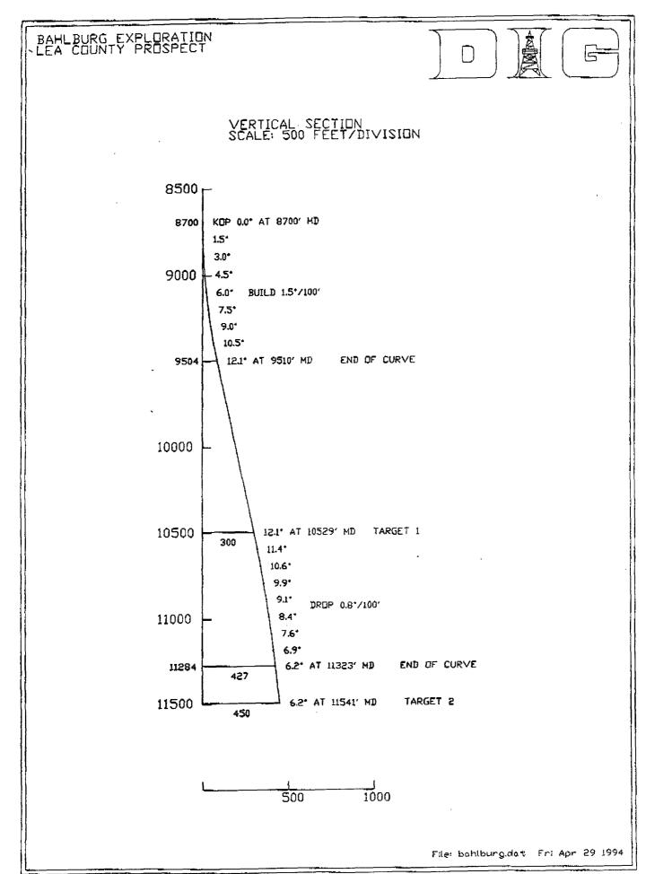
Figure 3. Planned sidetrack borehole trajectory in No.2 Harris well.
