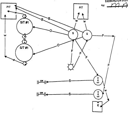
Attachment to the Site Facility Diagram - Lease NM General sealing of valves. Sales by tank gauging PRODUCTION PHASE: All drain valves and all sales valves are sealed closed.
