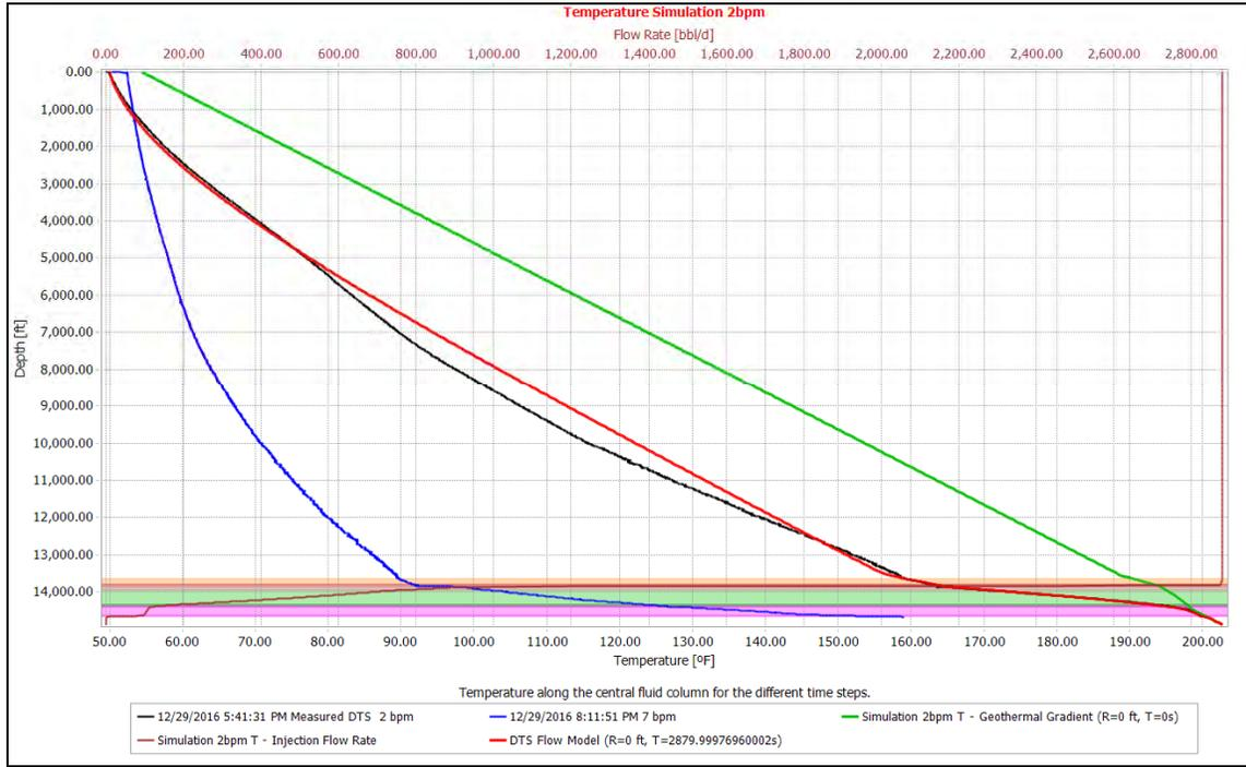
Figure 6: Thermal Simulation for Injection Distribution.
