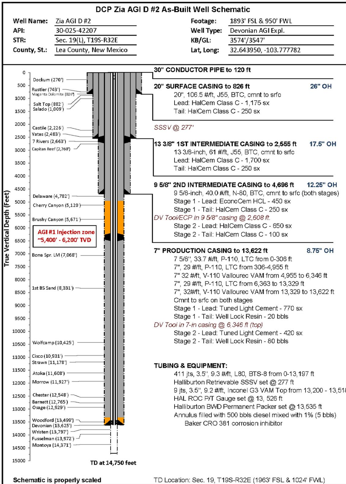
**FIGURE 3: Zia AGI D #2 as-built well schematic**
