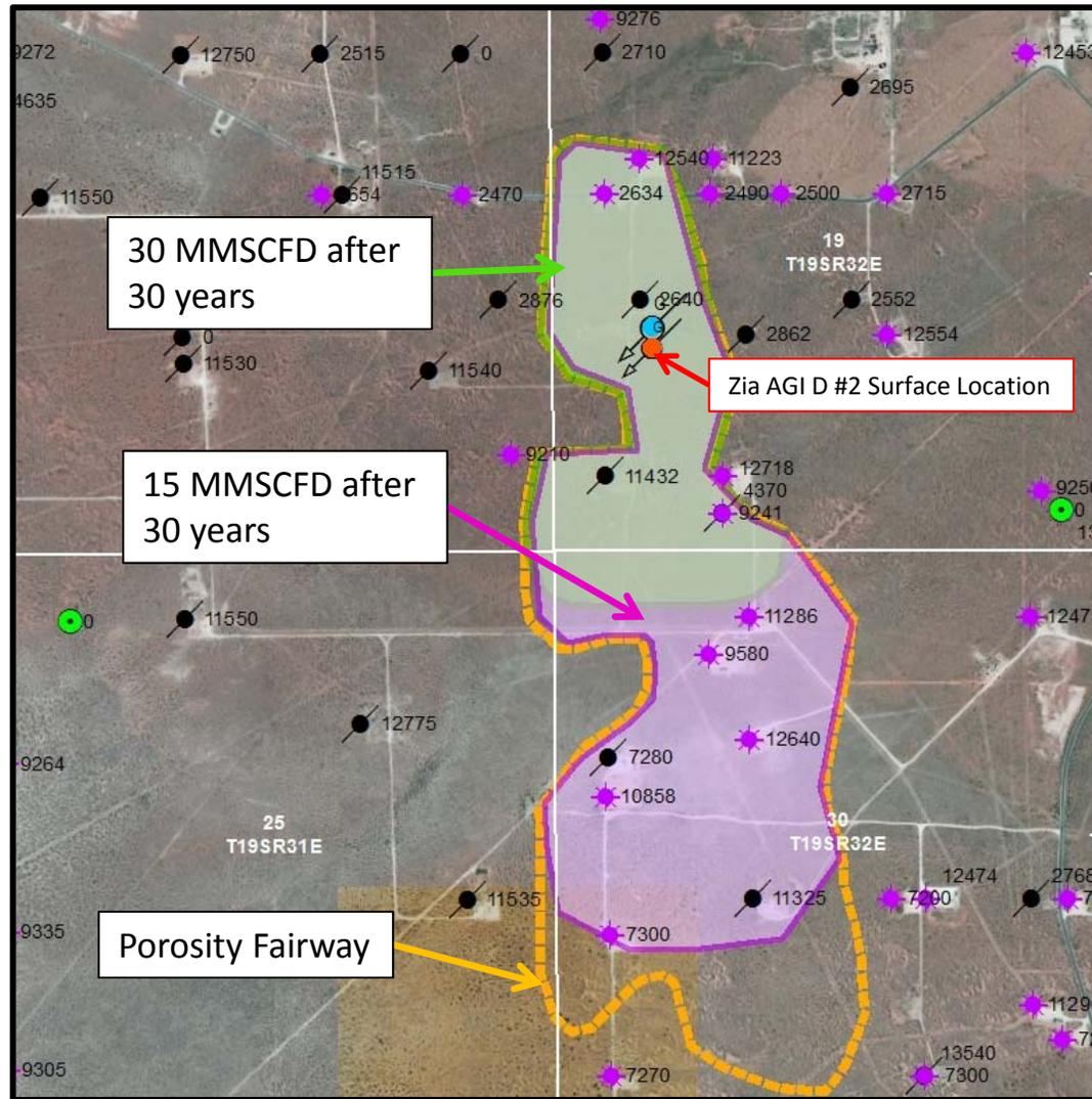
**FIGURE 12:** Porosity fairway in the Ordo-Devonian injection zone depicting migration of TAG plume after 30 years of injection
