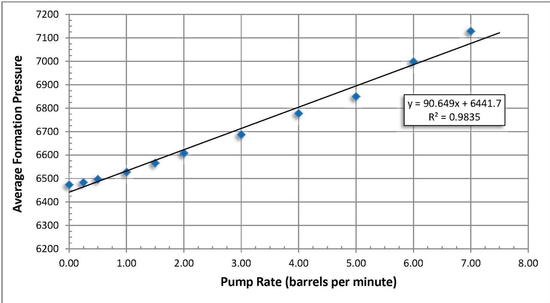
**FIGURE 17:** Formation Pressure at each step showing no break-over point, or parting pressure being reached within the injection zone.
