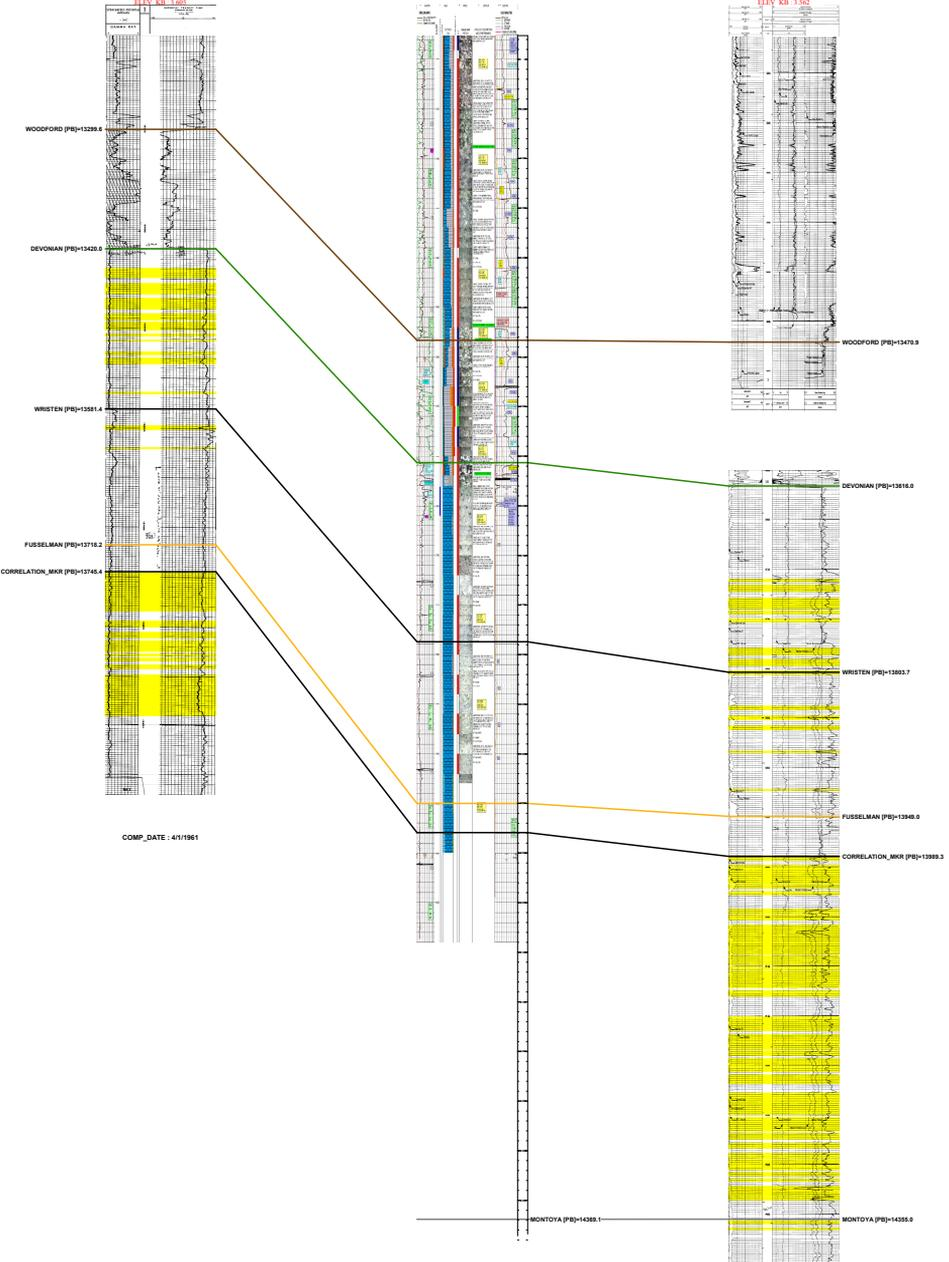
**Figure 11:** Cross section of the Ordo-Devonian injection zone and overlying Woodford shale caprock. Yellow highlights indicate high porosity.
