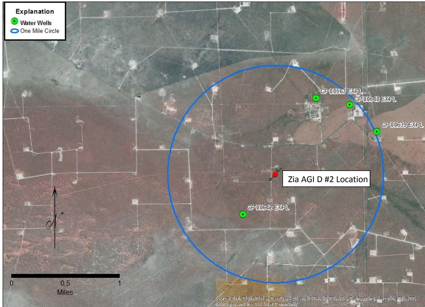
**FIGURE 13:** Water wells identified by the NM State Engineer’s files within one mile of Zia AGI D #2
