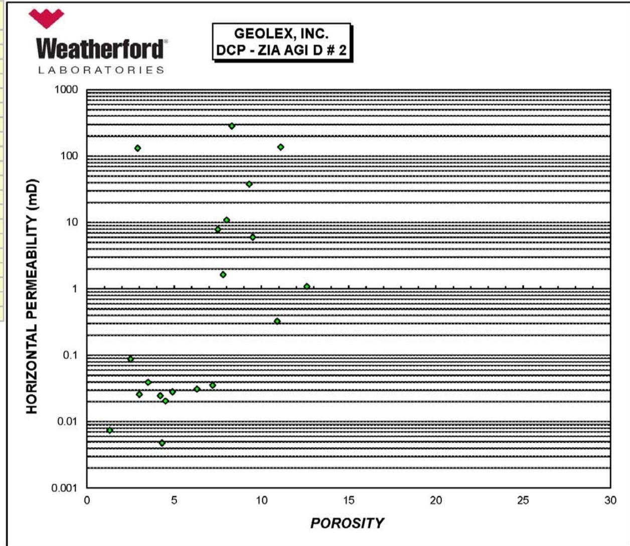
**Figure 15:** Porosity versus permeability from sidewall cores within the injection zone
