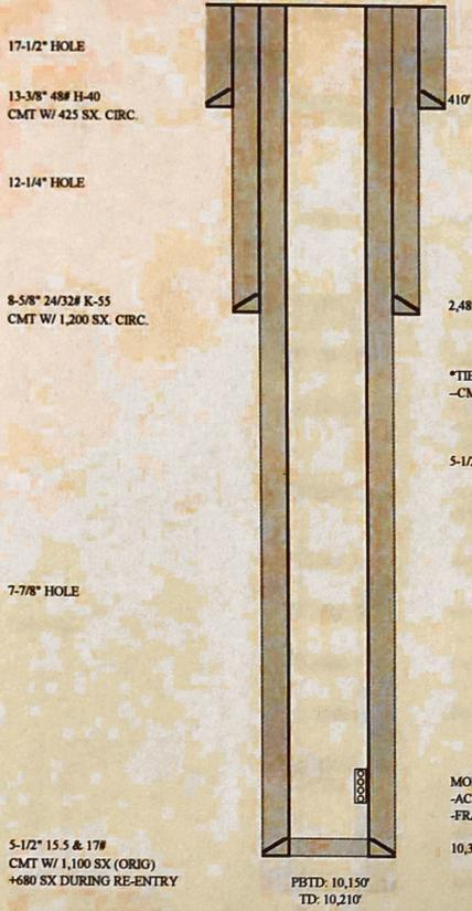
\*TIE INTO ORIGINAL 5-1/2" CSG @ 4,590' DURING RE-ENTRY
