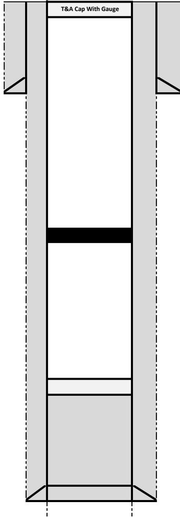
20" 94# J-55 Conductor Casing set @ 80' GL
