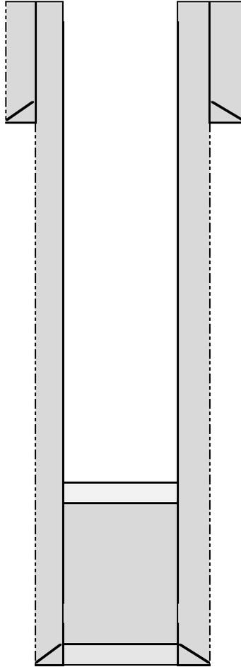
20" 94# J-55 Conductor Casing set @ 80' GL
