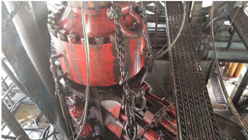
Figure 1: Winch System attached to BOP Stack
