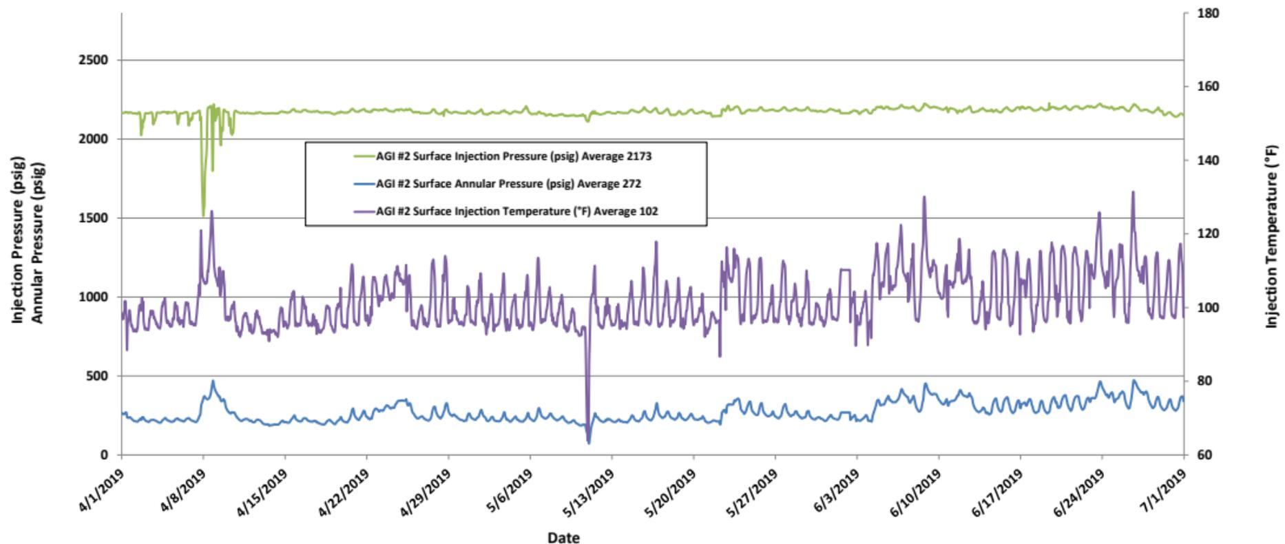
Figure 4: Maljamar AGI #2 BH Injection Pressure & Temperature, Surface Annular Pressure
