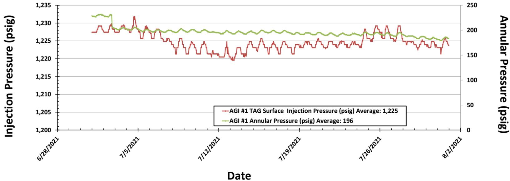
**Figure #3: Linam AGI #1 TAG Injection Pressure, Casing Annulus Pressure and TAG Injection Temperature**
