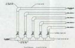
THERMAL OXIDIZER MANIFOLD DETAIL-TYPICAL
