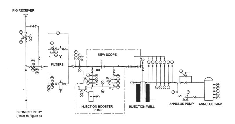
NOTE: All existing except as noted in red box. The 600 # ANSI flange on wellhead will be changed to 900 # ANSI. Booster pump installed on concrete pad with secondary containment to preclude release to environment.
