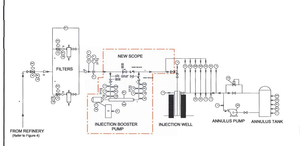
NOTE: All existing except as noted in red box. The 600 # ANSI flange on wellhead will be changed to 900 # ANSI. Booster pump installed on concrete pad with secondary containment to preclude release to environment.
