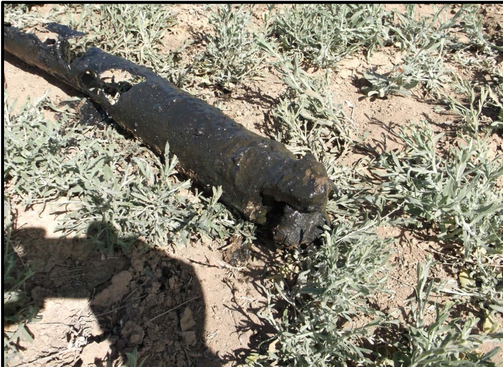
Photo 2: Driveshaft with yoke and u-joint retrieved from Jackson well.
