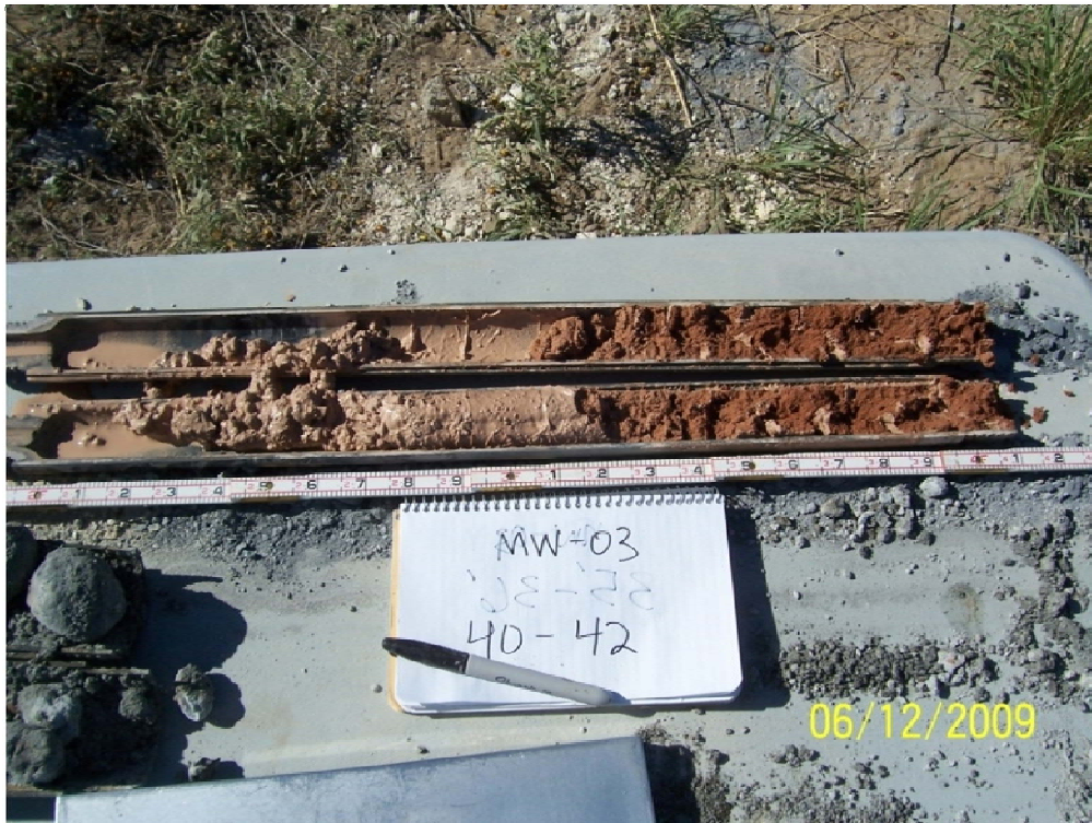
No. 5 – Soil core from MW-03 from 40-42 ft bgs; note the saturated soil.
