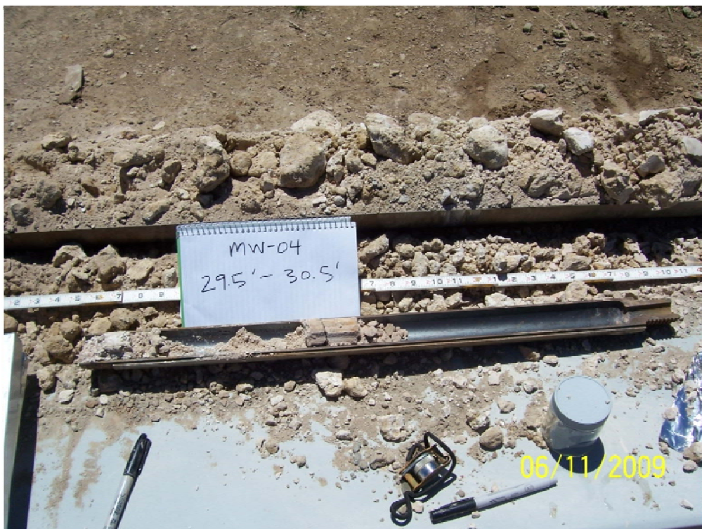
No. 6 – Soil core from MW-04 from 29.5- 30.5 ft bgs.
