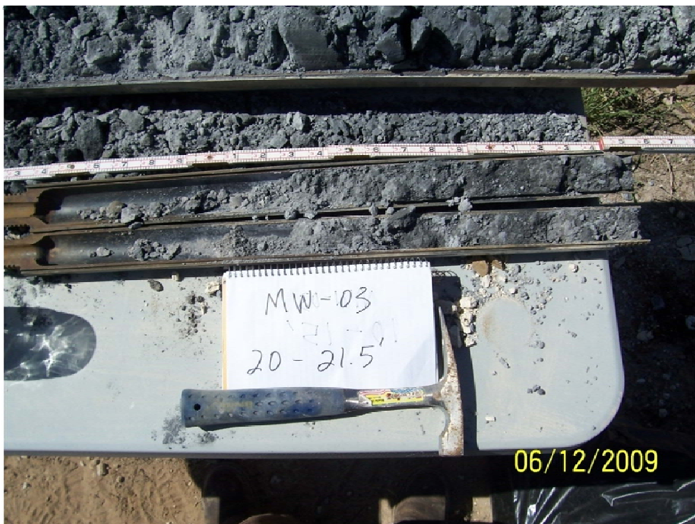
No. 4 – Soil core from MW-03 from 20-21.5 ft bgs; note the gray impacted soil.
