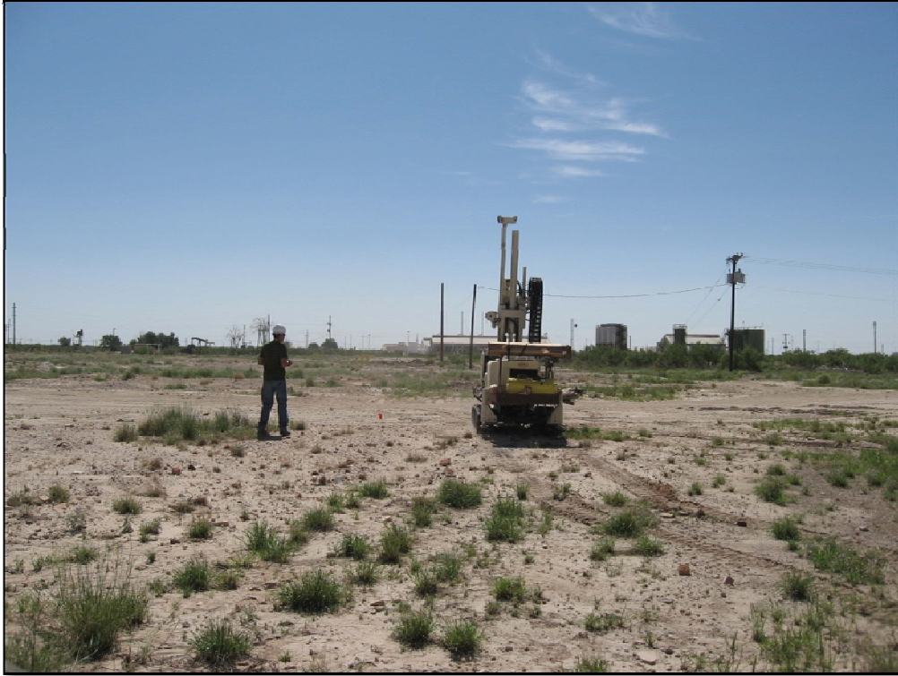
No. 13 – Direct Push Technology (DPT) rig used for DPB-01 through DPB-45.
