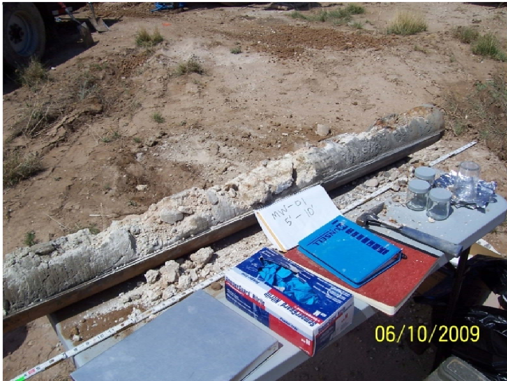
No. 1 – Soil core from MW-01 from 5-10 ft bgs.
