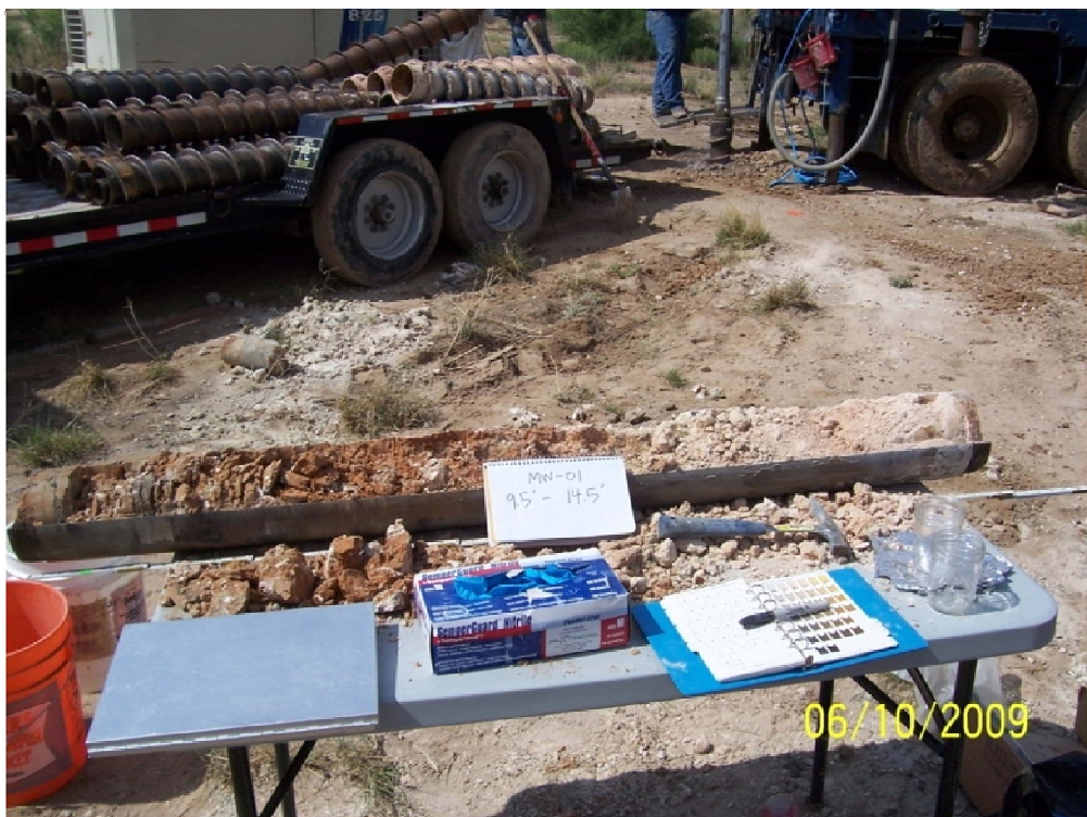
No. 2 – Soil core from MW-01 from 9.5-14.5 ft bgs; note the caliche.
