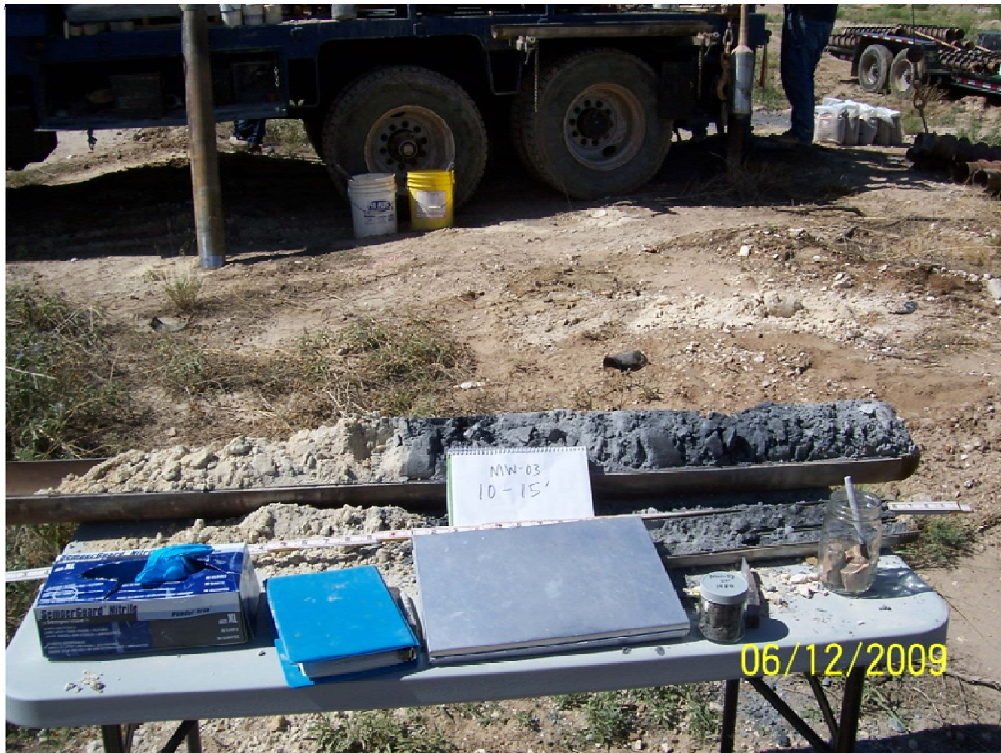
No. 3 – Soil core from MW-03 from 10-15 ft bgs; note the gray impacted soil.
