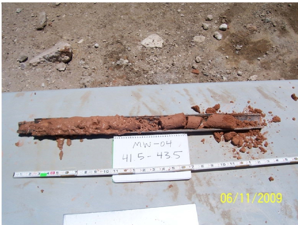
No. 8 – Soil core from MW-04 from 41.5-43.5 ft bgs; note the saturated soil.
