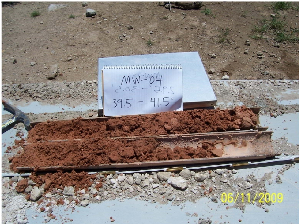
No. 7 – Soil core from MW-04 from 39.5-41.5 ft bgs; note wet clayey sand.
