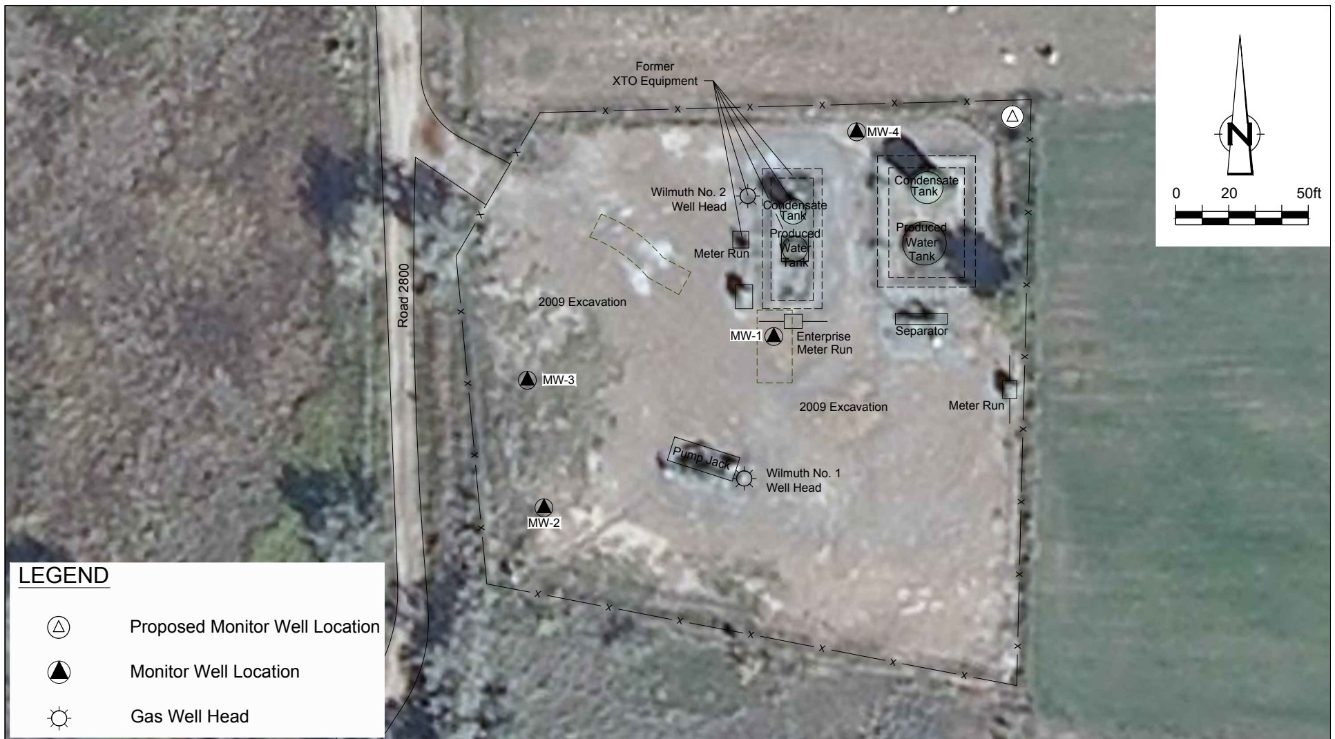
Figure 8 PROPOSED MONITOR WELL LOCATION MAP WILMUTH No. 1 NATURAL GAS WELL SITE SECTION 26, T31-R11W, SAN JUAN COUNTY, NEW MEXICO ConocoPhillips Company
