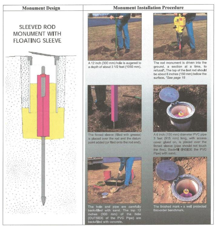
Attachment P - Subsidence Monument Rod Design and Installation Procedure
