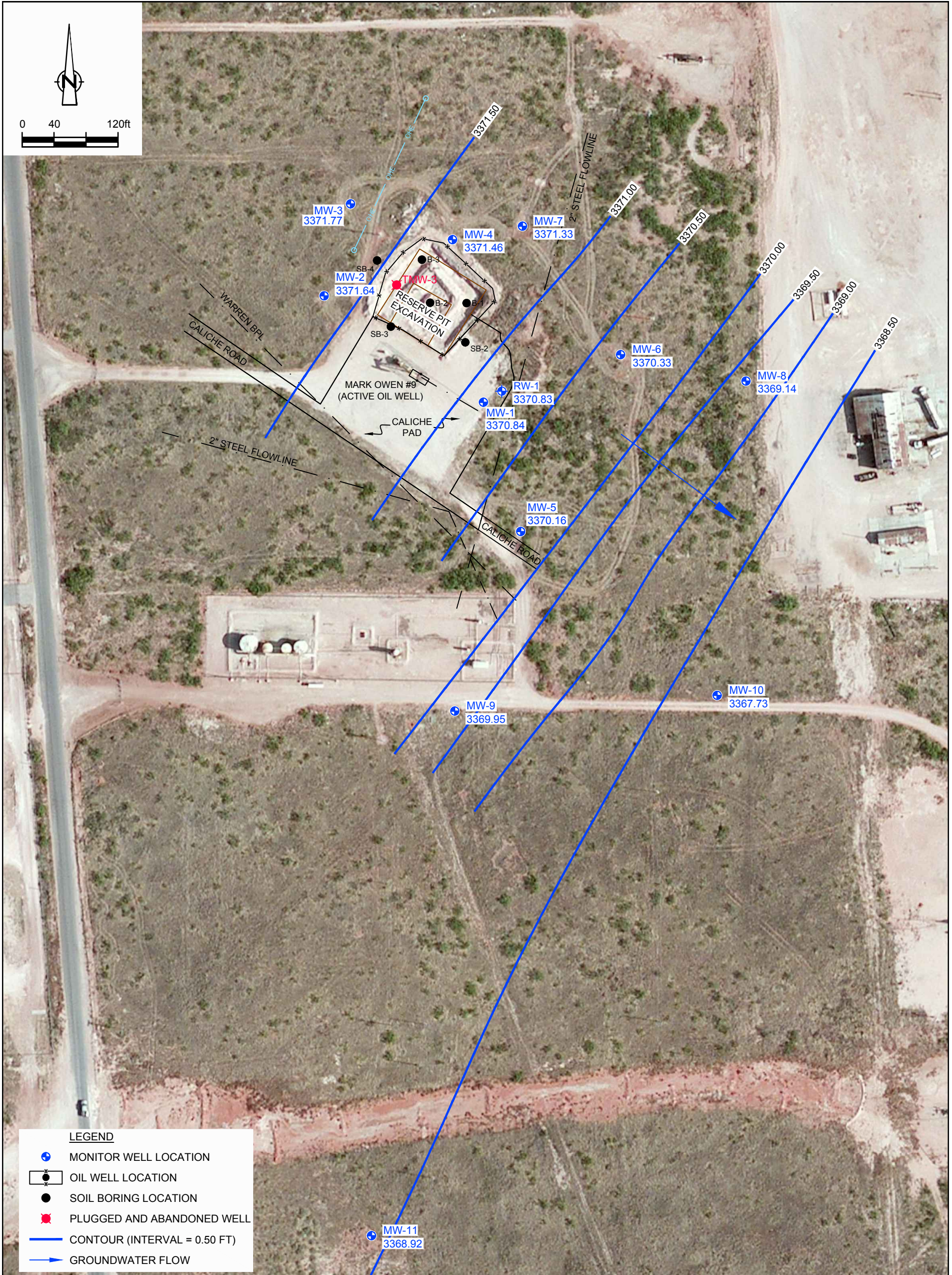
Figure 9 JUNE 2013 GROUNDWATER GRADIENT MAP MARK OWEN #9 RESERVE PIT NW/4 OF SE/4 SECTION 34; T-21-S, R-37-E LEA CO., NM Chevron Environmental Management Company
