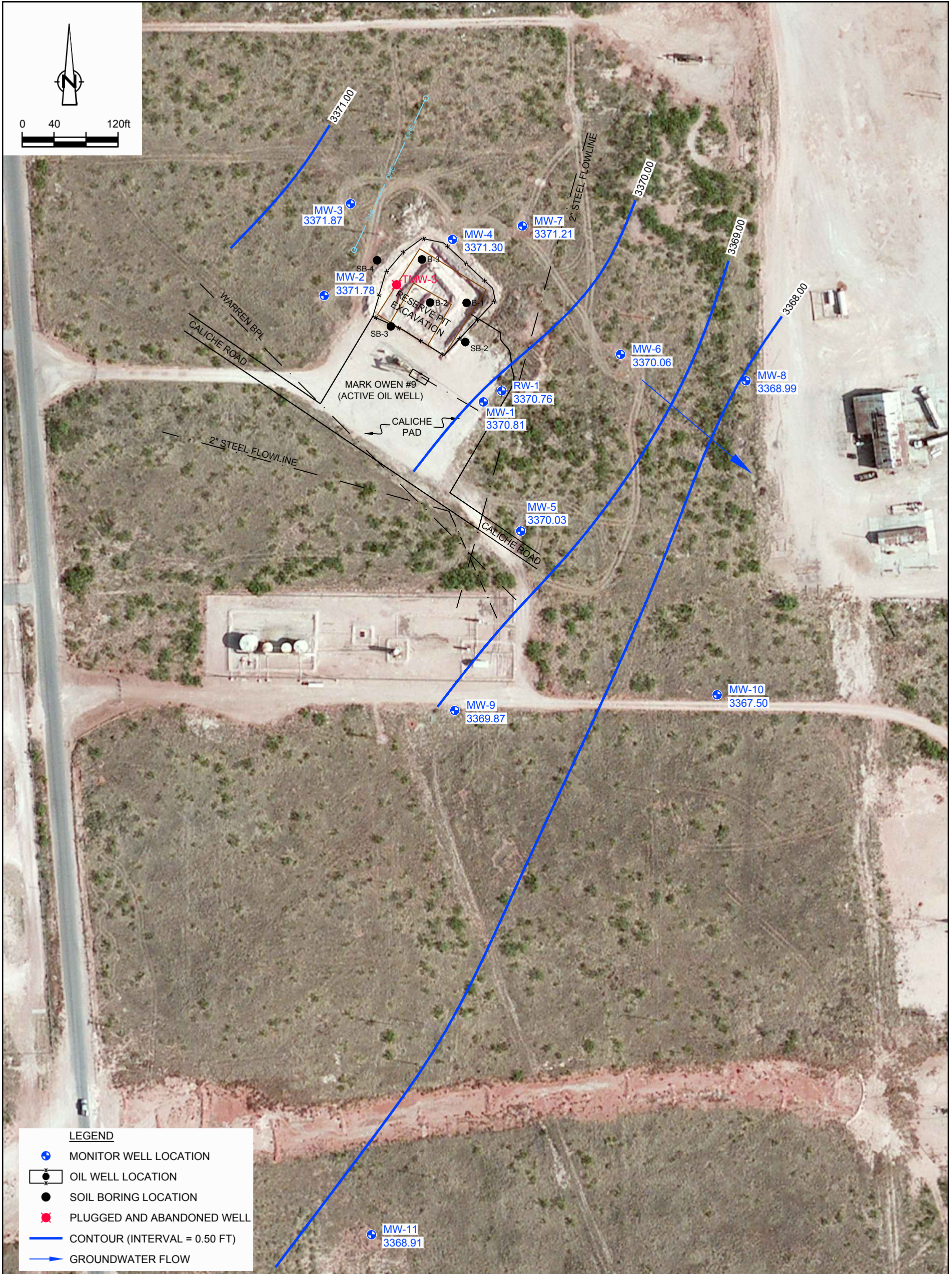
Figure 10 SEPTEMBER 2013 GROUNDWATER GRADIENT MAP MARK OWEN #9 RESERVE PIT NW/4 OF SE/4 SECTION 34; T-21-S, R-37-E LEA CO., NM Chevron Environmental Management Company
