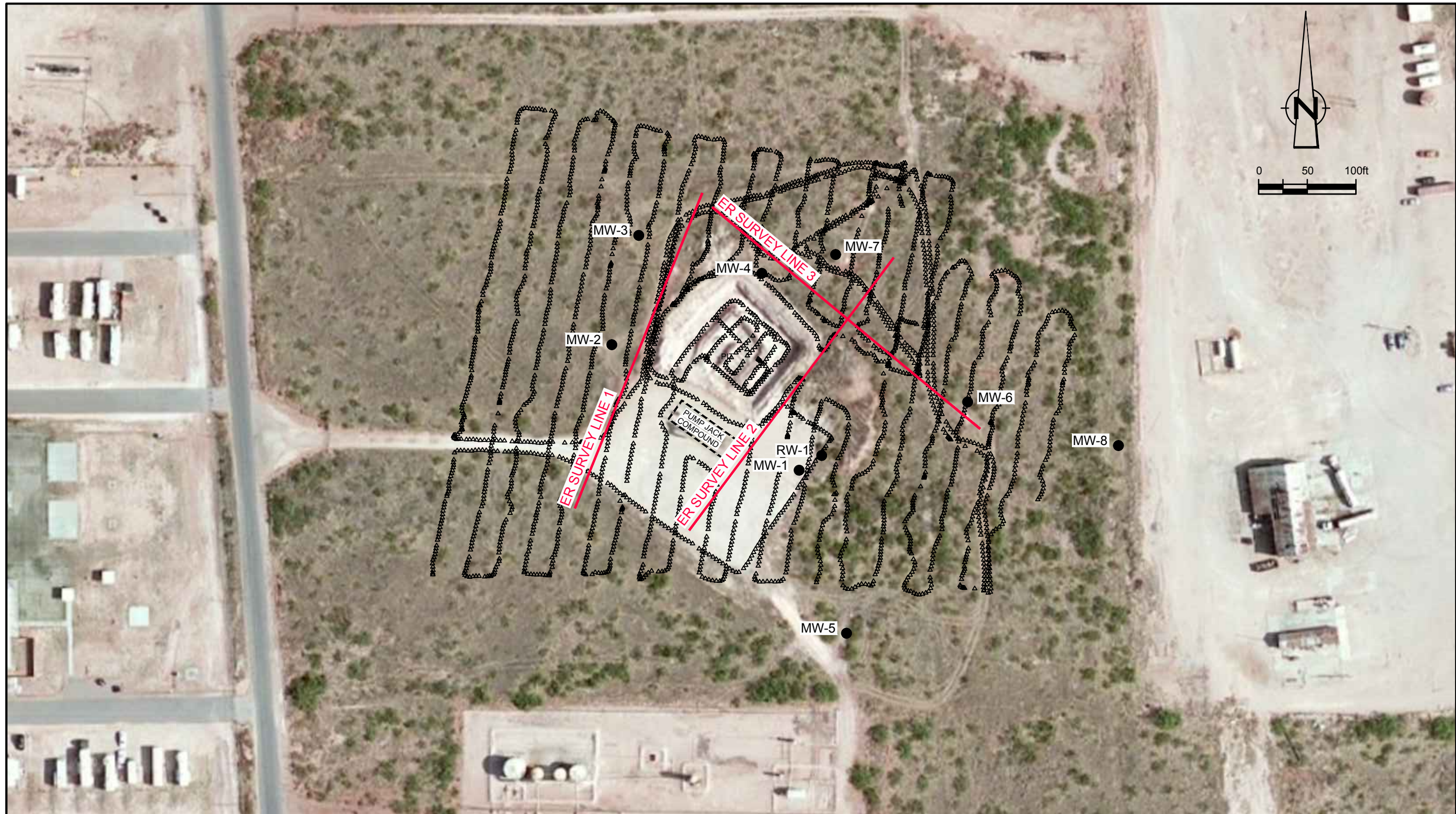
Figure 3 GEOPHYSICAL SURVEY COVERAGE MARK OWEN #9 RESERVE PIT CHEVRON ENVIRONMENTAL MANAGEMENT COMPANY Lea County, New Mexico
