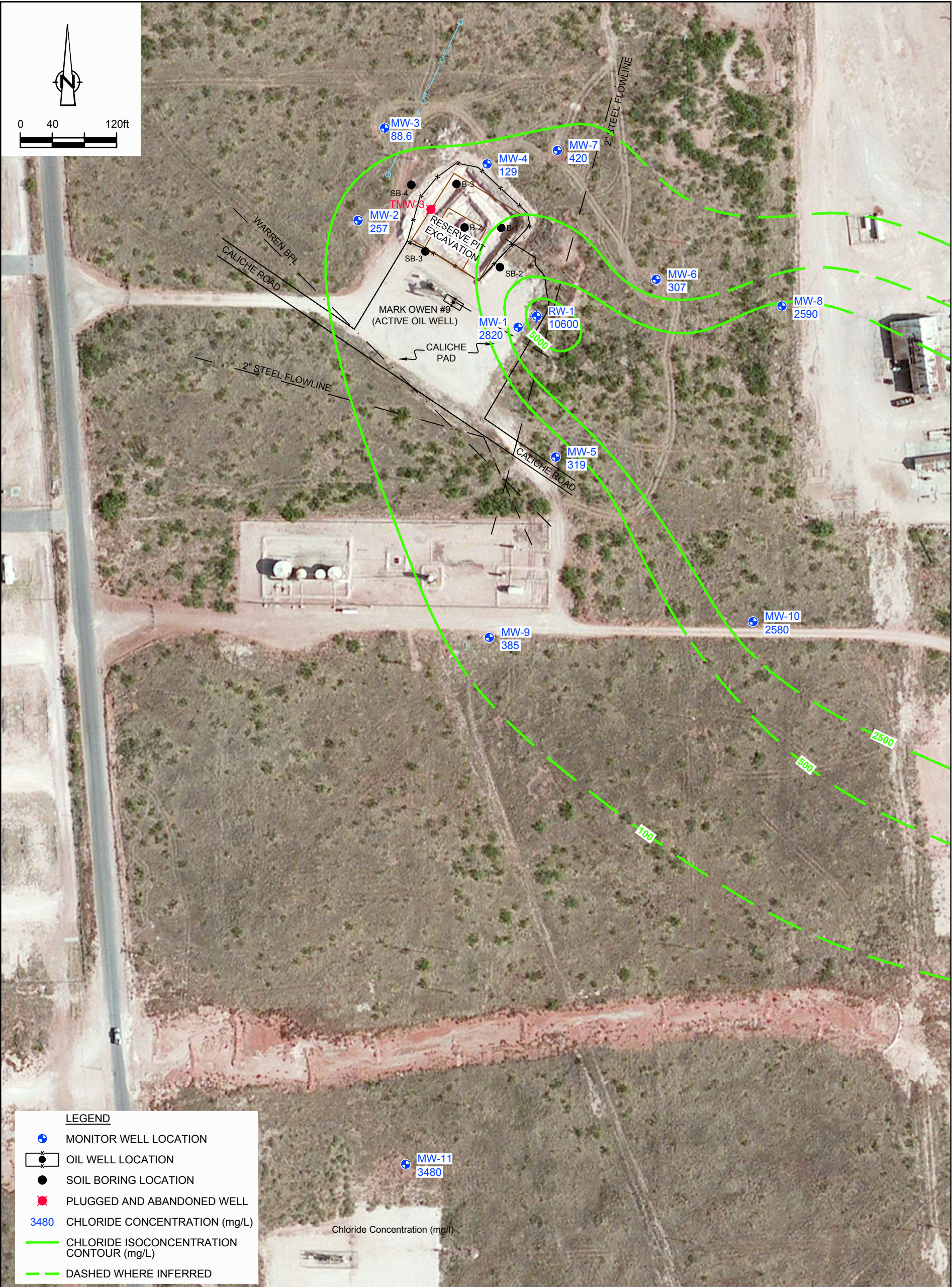
Figure 12 MARCH 2013 CHLORIDE CONCENTRATION MAP MARK OWEN #9 RESERVE PIT NW/4 OF SE/4 SECTION 34; T-21-S, R-37-E LEA CO., NM Chevron Environmental Management Company
