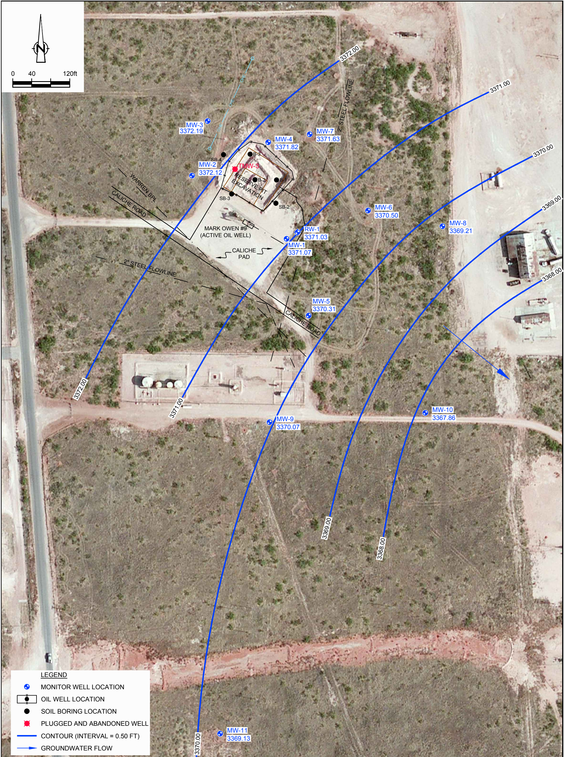
Figure 11 NOVEMBER 2013 GROUNDWATER GRADIENT MAP MARK OWEN #9 RESERVE PIT NW/4 OF SE/4 SECTION 34; T-21-S, R-37-E LEA CO., NM Chevron Environmental Management Company
