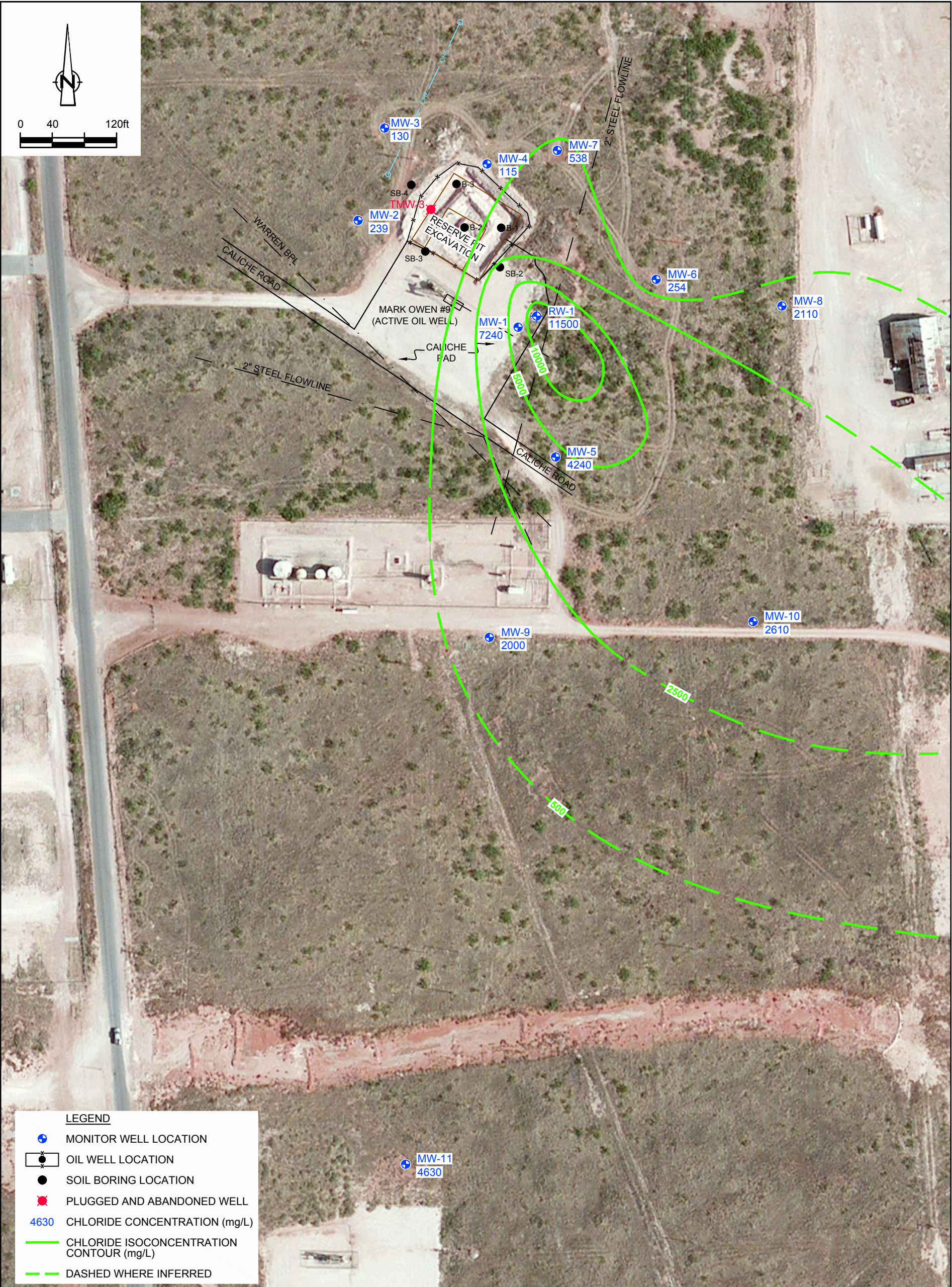
Figure 15 NOVEMBER 2013 CHLORIDE CONCENTRATION MAP MARK OWEN #9 RESERVE PIT NW/4 OF SE/4 SECTION 34; T-21-S, R-37-E LEA CO., NM Chevron Environmental Management Company
