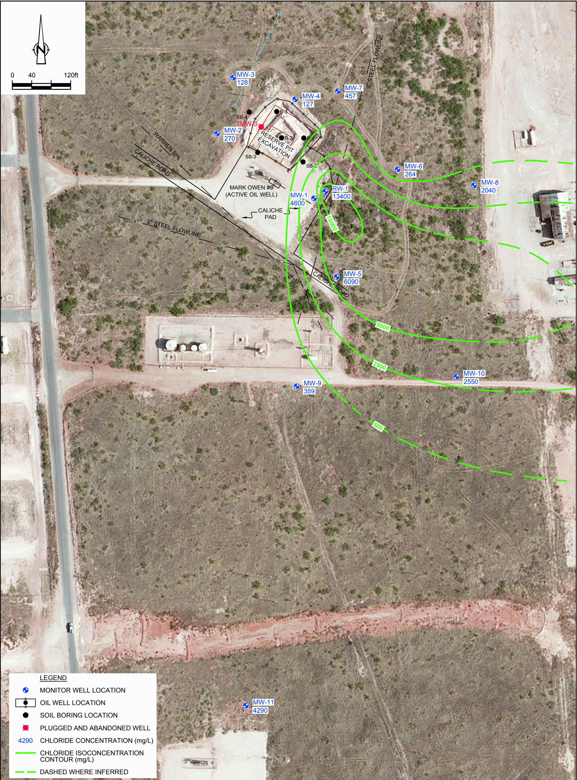
Figure 14 SEPTEMBER 2013 CHLORIDE CONCENTRATION MAP MARK OWEN #9 RESERVE PIT NW/4 OF SE/4 SECTION 34; T-21-S, R-37-E LEA CO., NM Chevron Environmental Management Company
