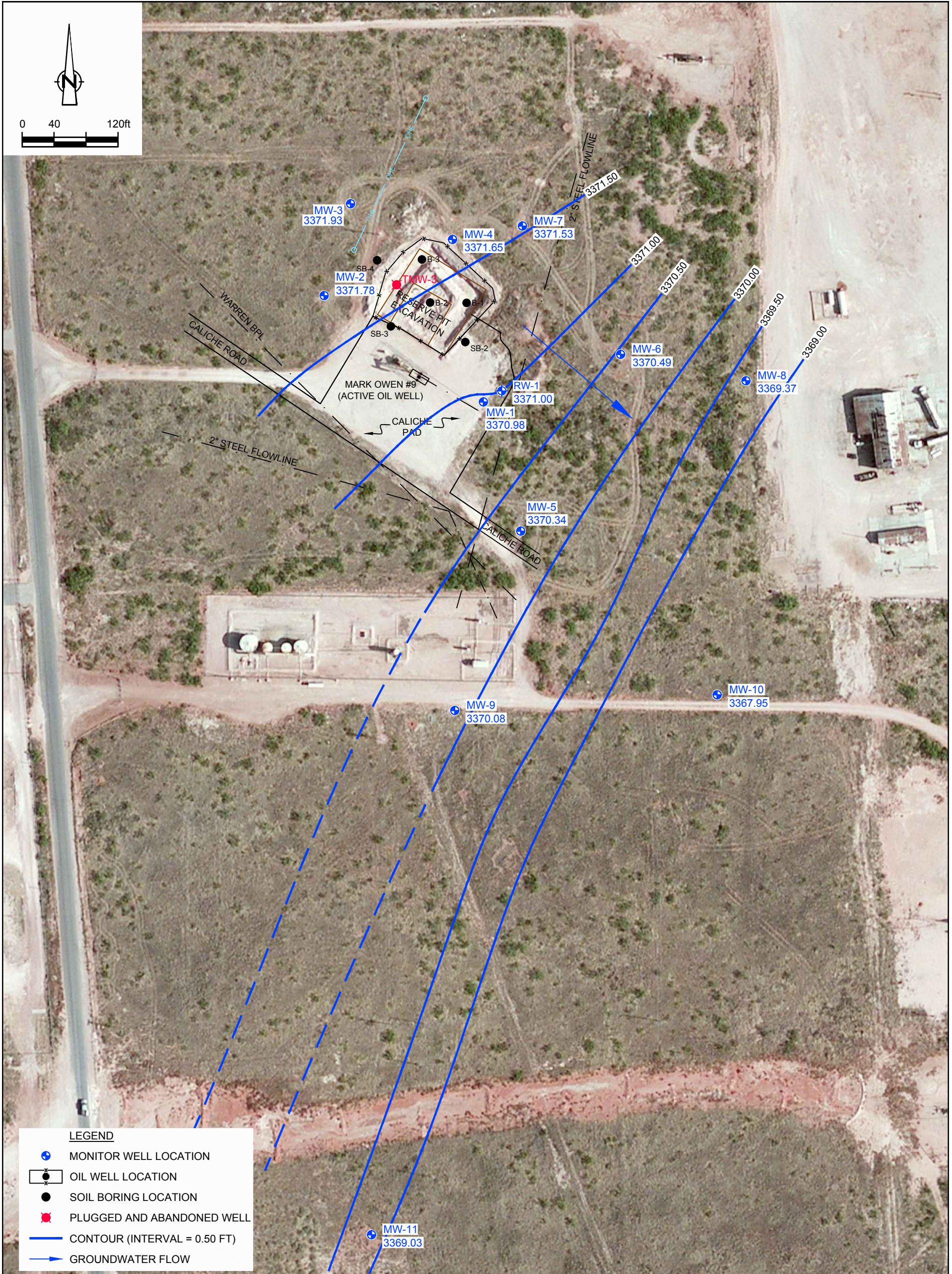
Figure 8 MARCH 2013 GROUNDWATER GRADIENT MAP MARK OWEN #9 RESERVE PIT NW/4 OF SE/4 SECTION 34; T-21-S, R-37-E LEA CO., NM Chevron Environmental Management Company
