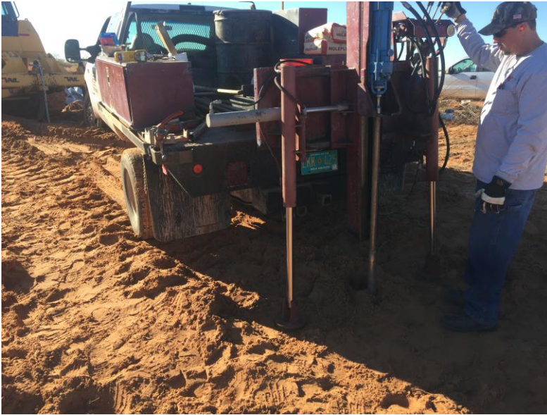
Photo 1: View of a typical boring installed via geoprobe.
