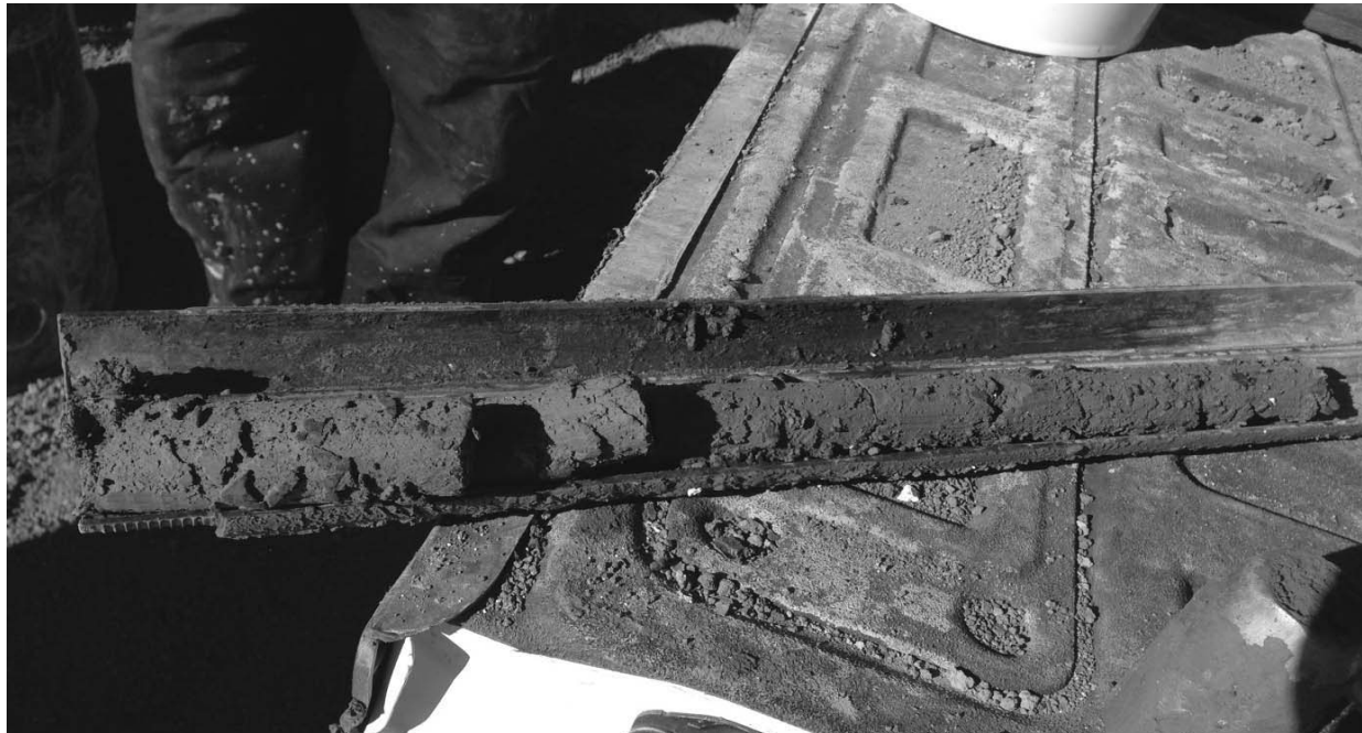
Bottom of Split Spoon Sample from 12 to 14 Feet Deep
