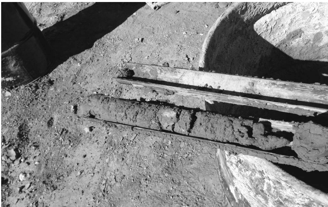
Bottom of Split Spoon Sample from 4 to 6 Feet Deep
