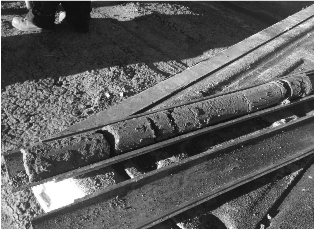
Bottom of Split Spoon Sample from 2 to 4 Feet Deep
