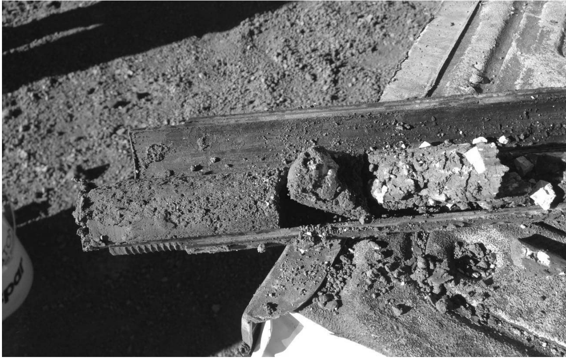
Bottom of Split Spoon Sample from 8 to 10 Feet Deep
