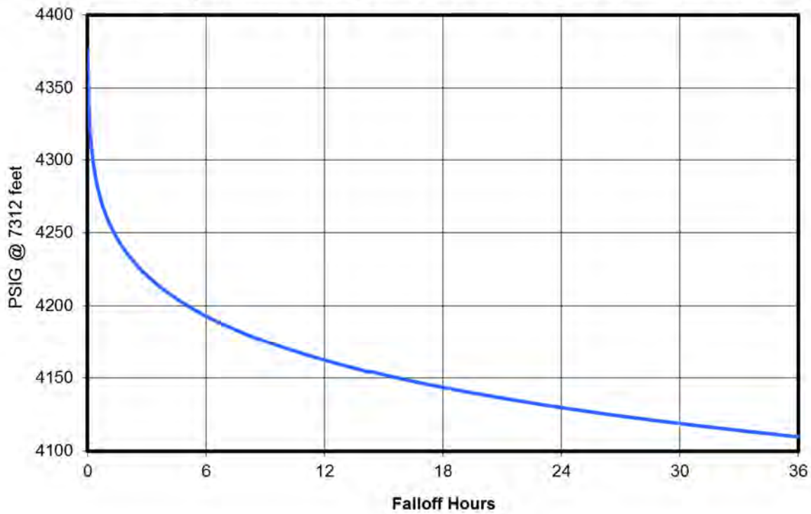
Figure 3 Disposal Well #2 - October 5, 2017 FO Test
