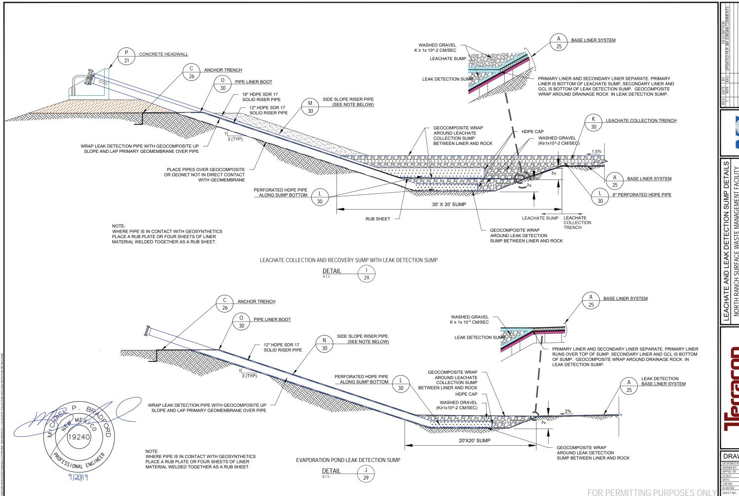
LEACHATE AND LEAK DETECTION SUMP DETAILS
