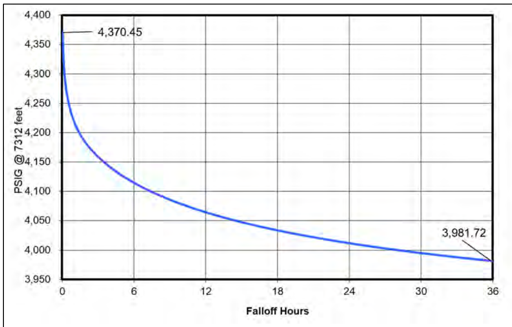
Figure 3 – Pressure vs Time for the Early Part of the Falloff Test.
