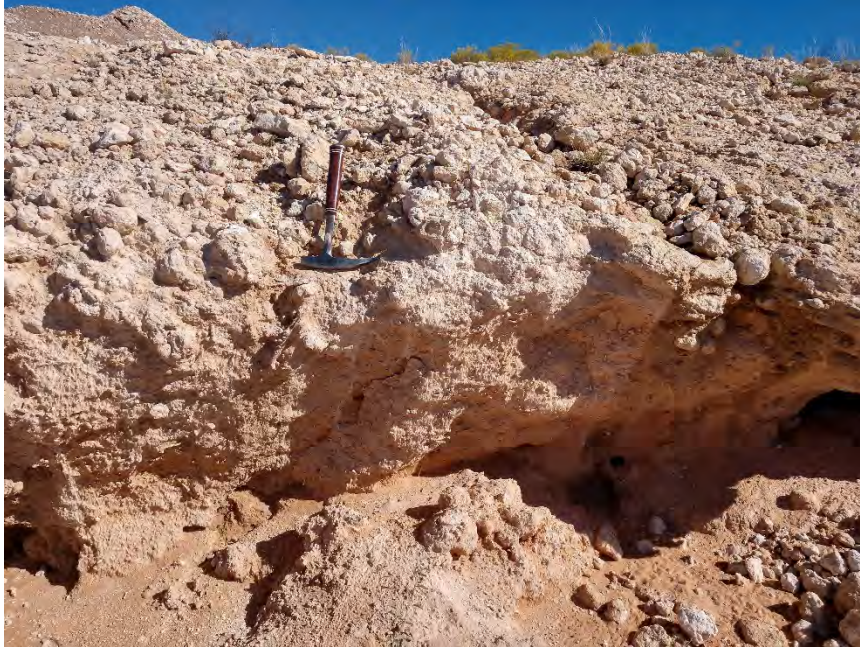
Figure 2: Calcrete caprock ~six feet thick overlying poorly indurated alluvial material near proposed Superman recycling facility.
