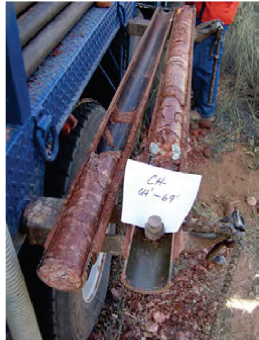
Photograph 14. Core sample of claystone with grey clay inclusions (Chinle) in CH-2.
