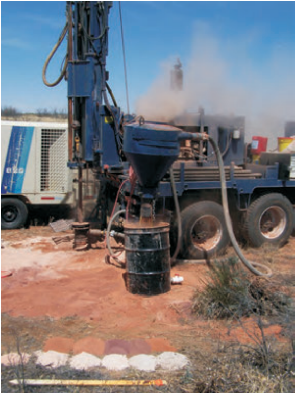
Photograph 17. Rodgers drilling dry Chinle Formation at MP-4 using air rotary.
