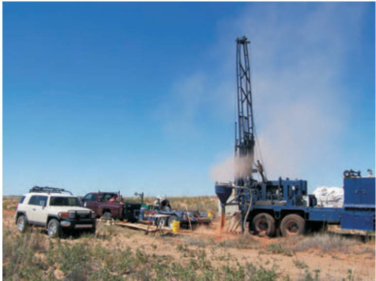
Photograph 15. Rodgers set up on MP-3 with CME-75 combination HSA and air rotary drill rig and related equipment.
