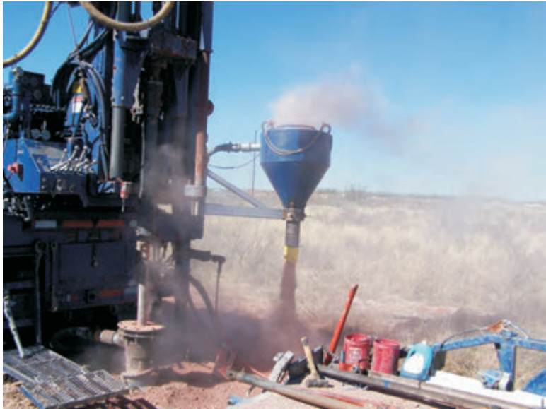
Photograph 12. Air rotary drilling dry Chinle Formation at MP-2.
