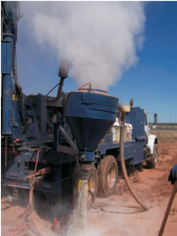
Photograph 14. Air rotary drilling dry Chinle Formation at MP-3.
