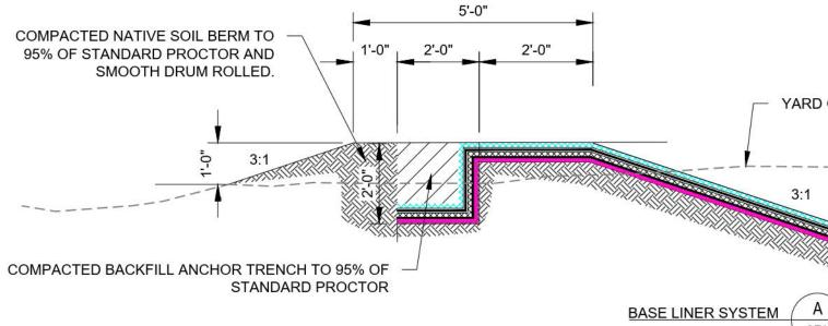
EVAPORATION POND CONTAINMENT BERM AND ANCHOR TRENCH
