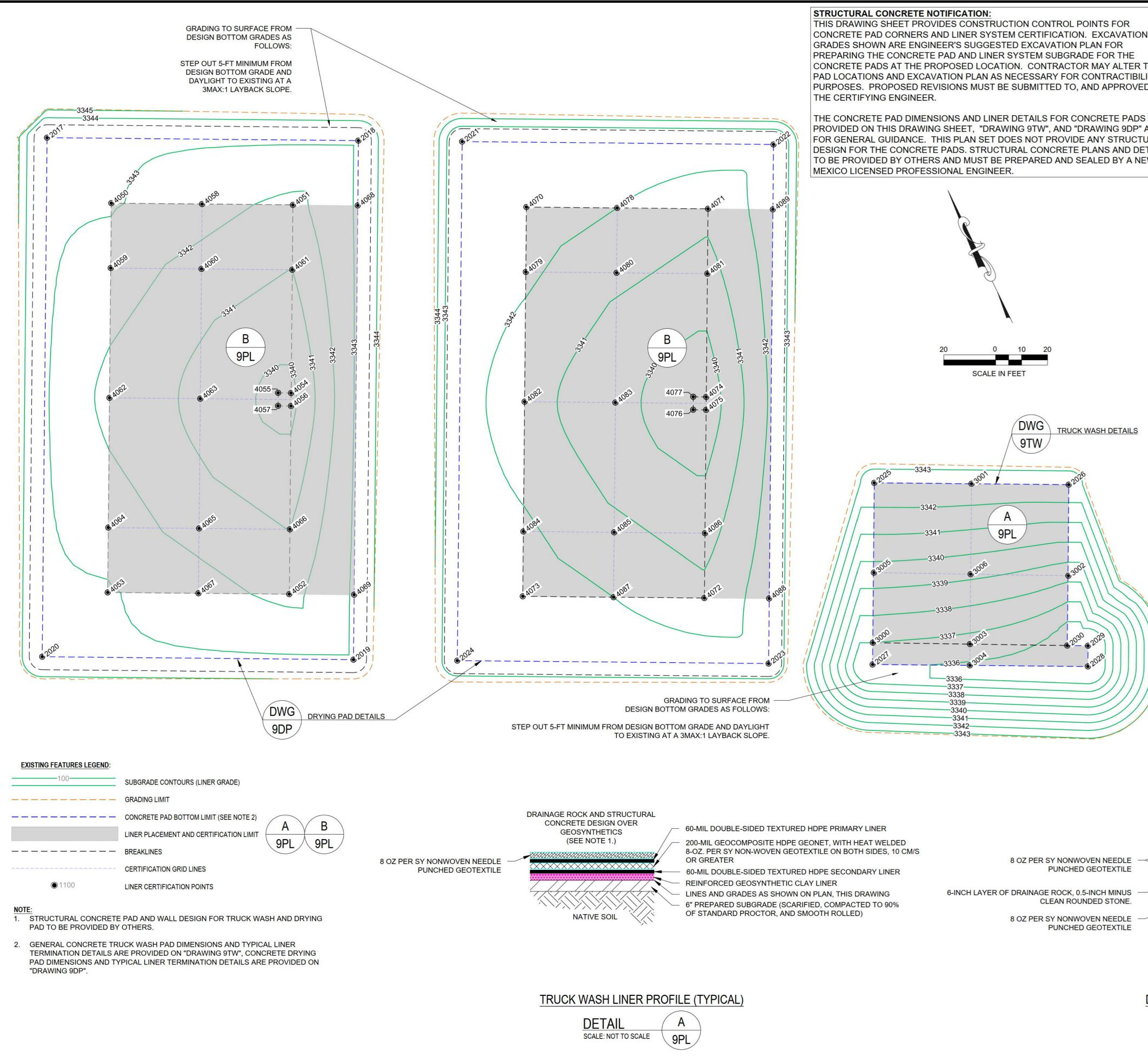
CONCRETE PAD CORNERS AND LINER SYSTEM CERTIFICATION. EXCAVATION CONCRETE PADS AT THE PROPOSED LOCATION. CONTRACTOR MAY ALTER THE PAD LOCATIONS AND EXCAVATION PLAN AS NECESSARY FOR CONTRACTIBILITY PURPOSES. PROPOSED REVISIONS MUST BE SUBMITTED TO, AND APPROVED BY
