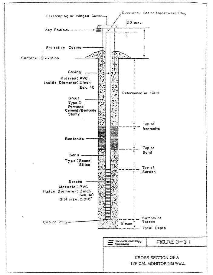
The volume of filter material needed to fill the annular space will be calculated. Bridging of materials has occurred if less than the calculated volume is needed to fill the space. If this occurs, a tremie pipe may be used to break the bridging and correctly fill the space.
