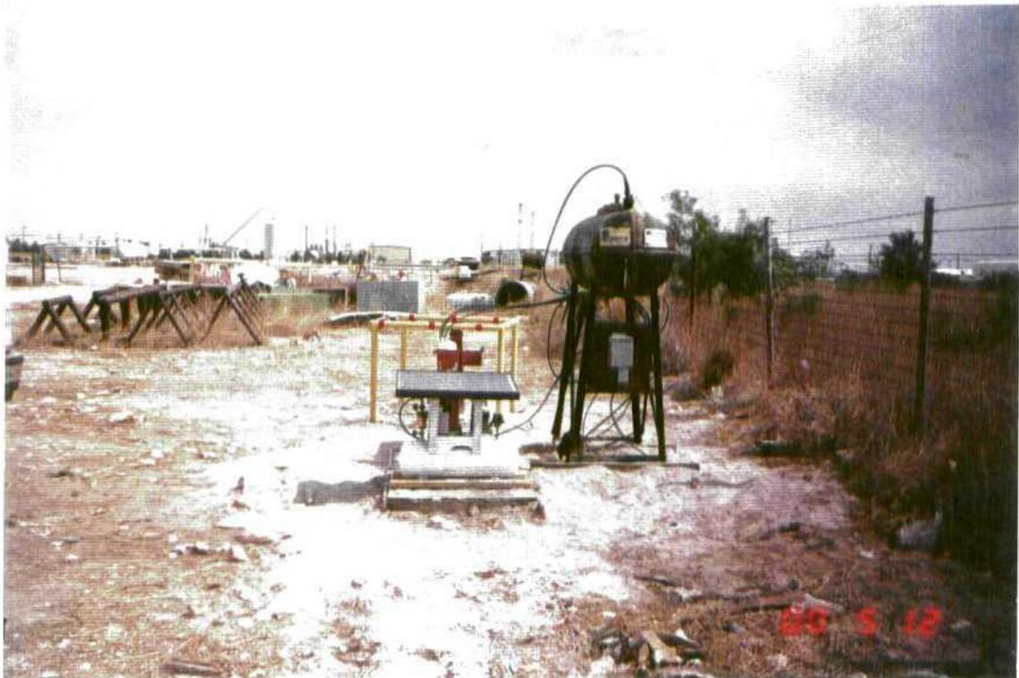
View facing north showing Xitech product recovery system installed at recovery well RW-1.
