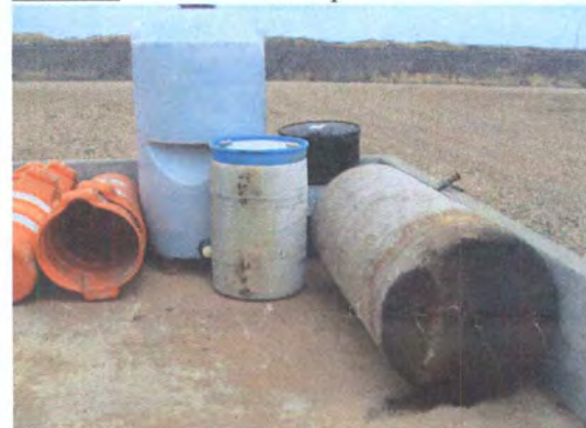
Photo 6 : Containers within secondary containment.
