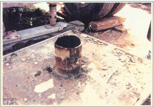
Test perforation at surface
