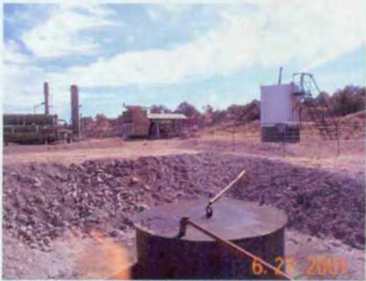
Pic #2 looking ENE- Water overflow tank; background shows compressor, condensate & water tank, and pipeline de-hydration equipment.
