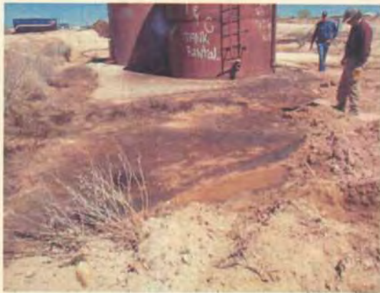
oil soaked soil observed around old storage tank area. Berms were built out of contaminated soil.
