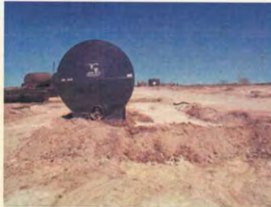
Area between shop and frac tank wash-out area. New berms were constructed out of contaminated soil. No liner under new tank.
