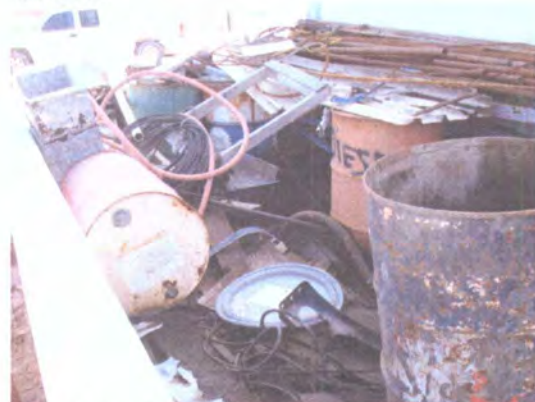
Photo 5: Open top barrels, housekeeping concern. Barrels not labeled.
