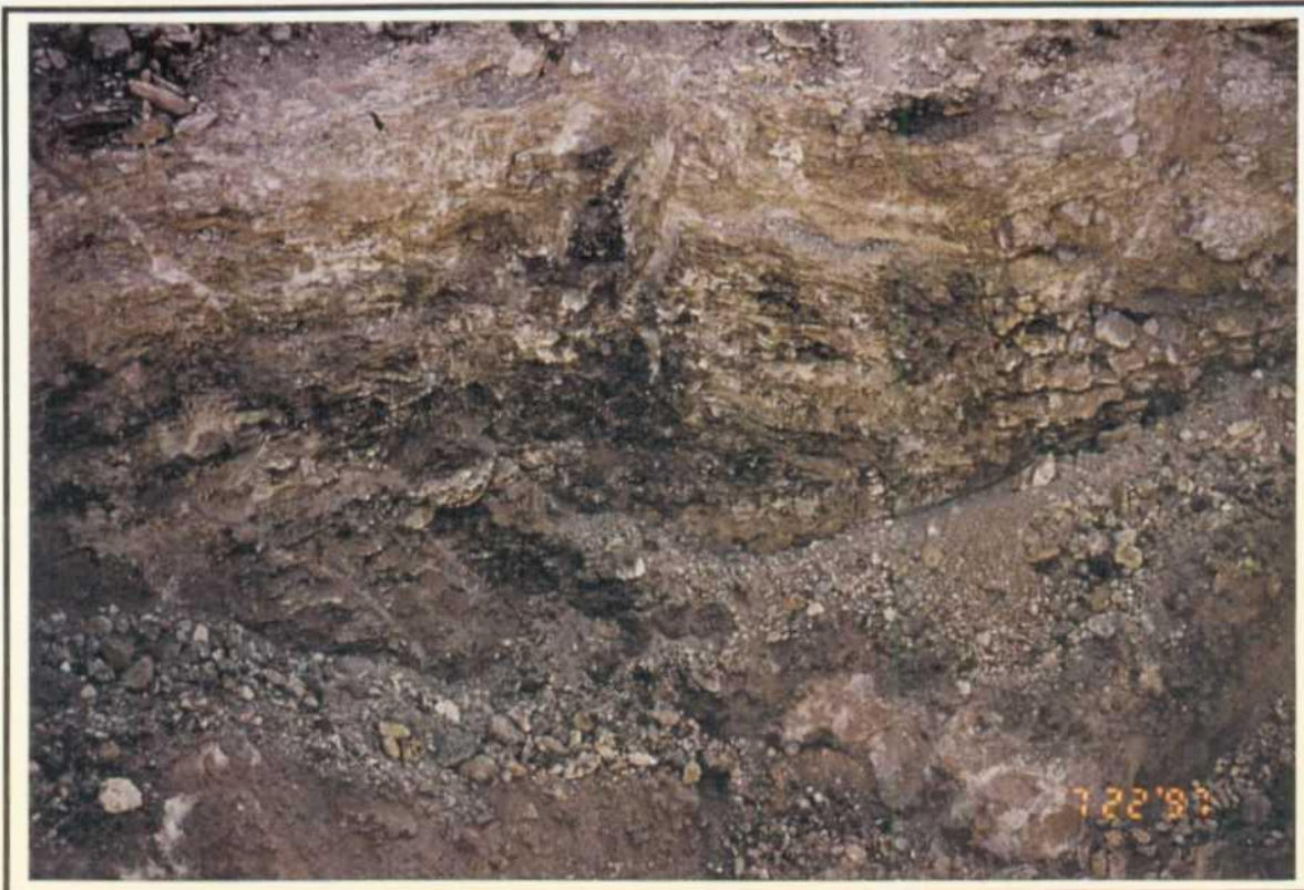
Photo 31: Typical hydrocarbon impacted soil at mechanics pit/leach field.
