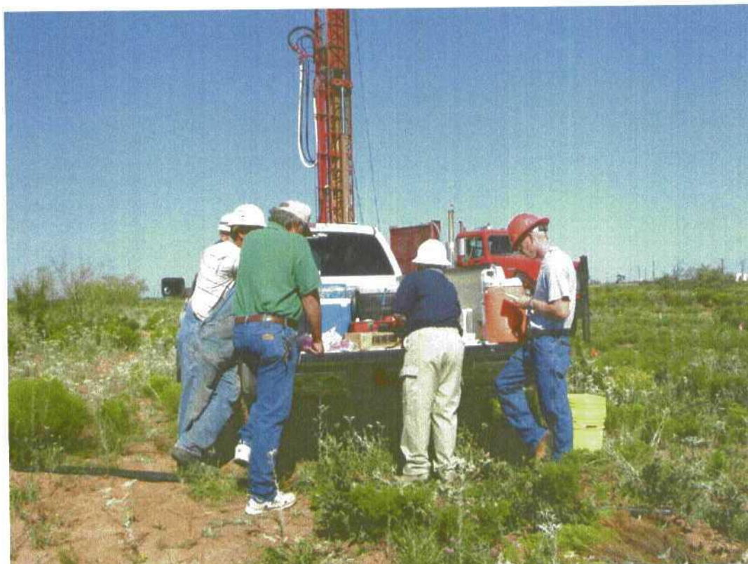
View facing west showing chloride screening activities for soil samples obtained from monitoring well MW-1 at the Santa Rita EOL site (08-30-06)
