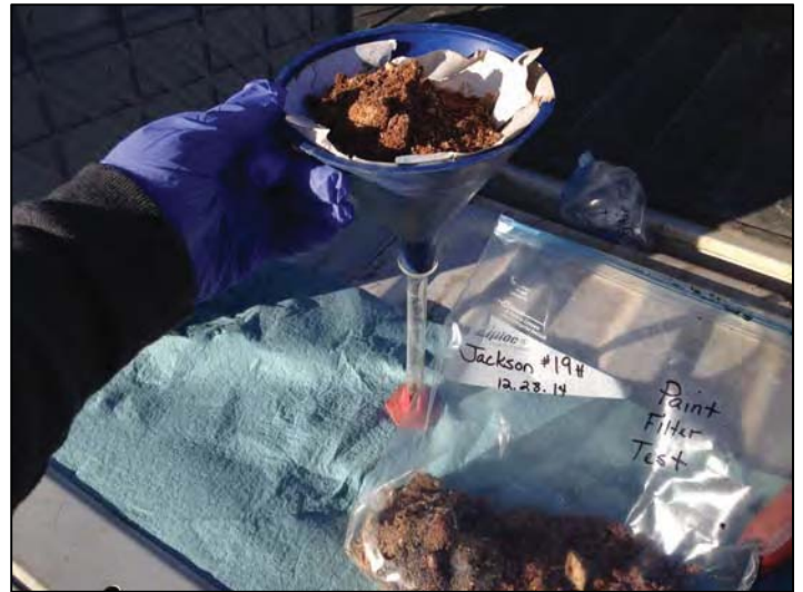
Paint filter test on stabilized cuttings 12/28/2014
