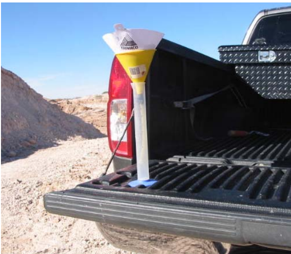
Figure 2 : Paint Filter Test at Harris #1, October 14, 2014.
