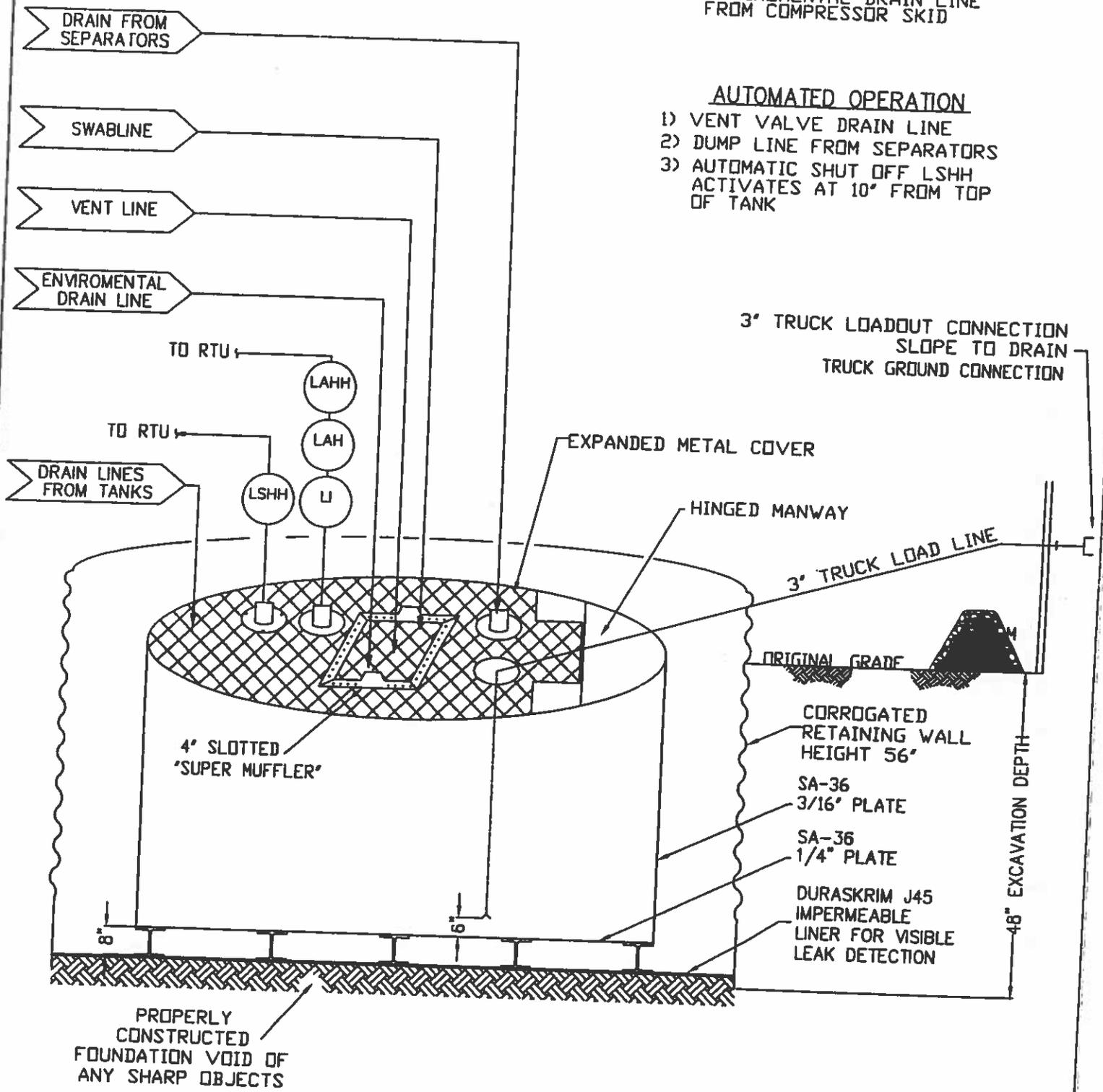
3" TRUCK LOADOUT CONNECTION
