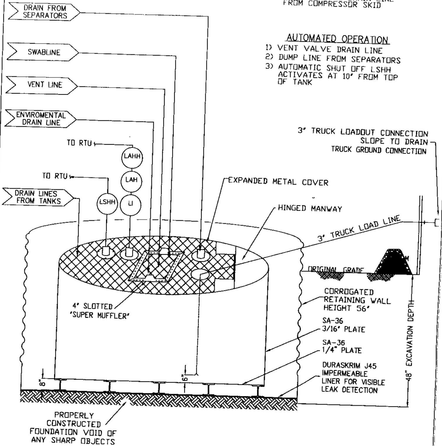
3" TRUCK LOADOUT CONNECTION
