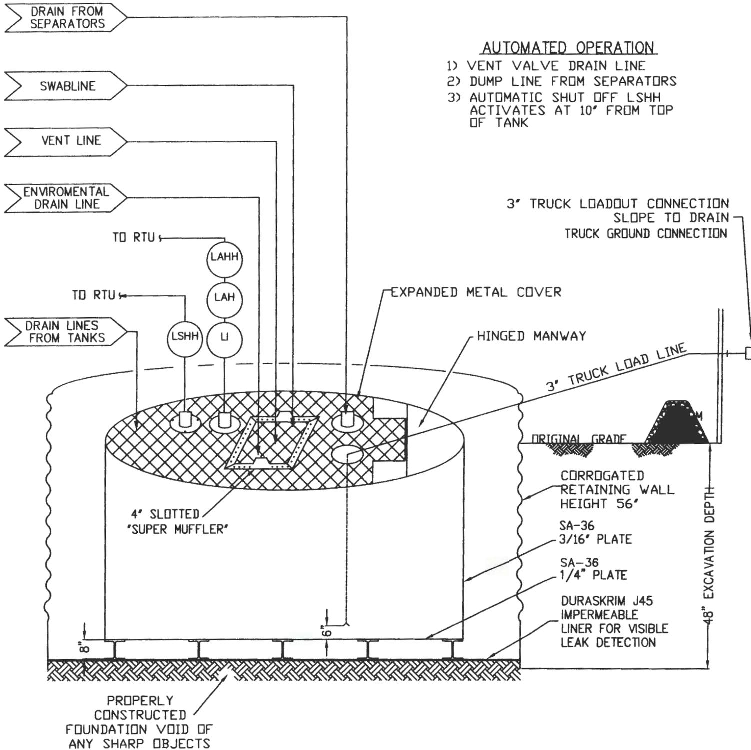
3" TRUCK LOADOUT CONNECTION
