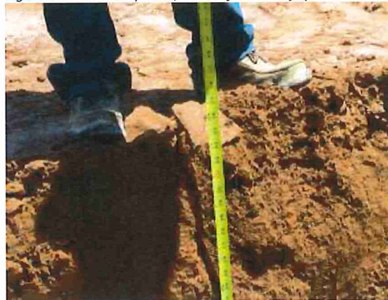
Figure 5 32-inch deep hole, West of Center of spill
