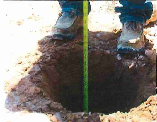
Figure 4 29-inch deep hole, South edge of spill
